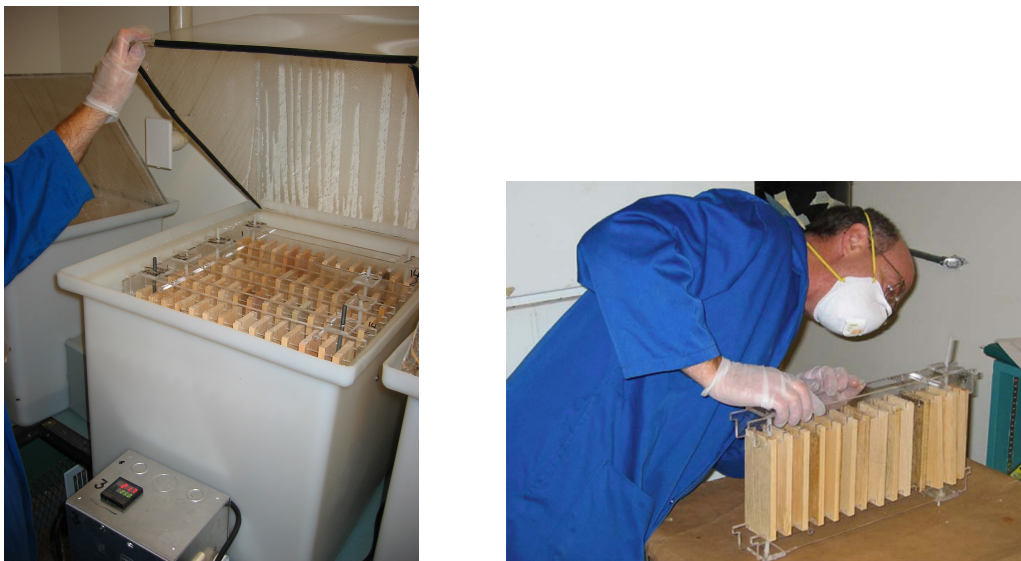
Figure 1. Samples in the test chamber being tested for mold resistance (left); and assessment and rating of mold growth (right)
