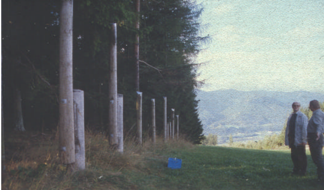
Fig. 12: Spruce poles treated with Trichoderma harzianum planted in soil and screwed on mast feet, respectively.
