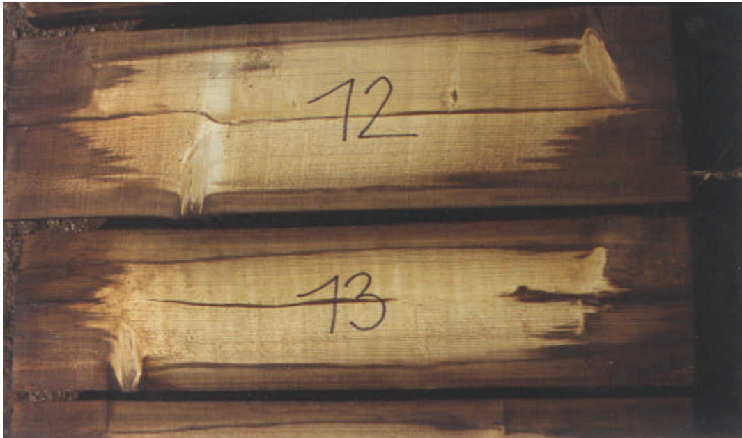
Fig. 8: Penetration of creosote after pre-treatment with Dichomitus squalens . The selected basidiomycetes also effected heartwood penetration.
