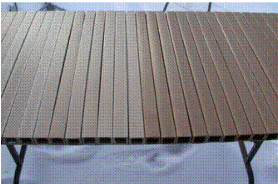
Figure 1. Extruded profiles of natural fiber plastic composites exposed in the short- and long-term tests.
