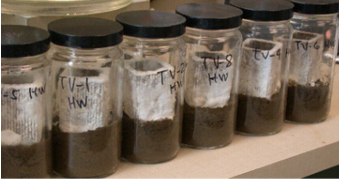
Figure 7. Trametes versicolor growing on blocks of a natural flour plastic composite in a soil block test.
