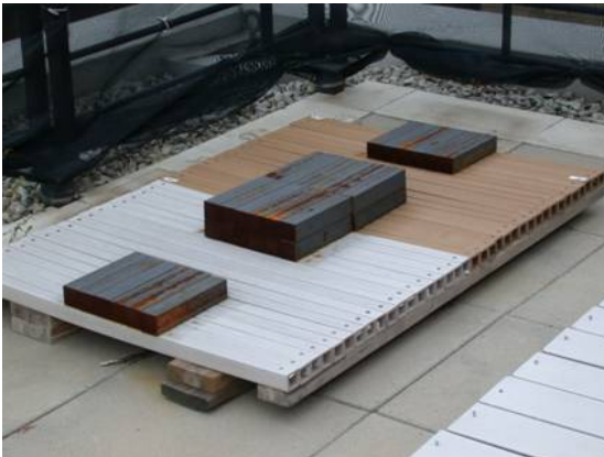
Figure 3. Specimens of natural fiber plastic composites exposed to exterior weathering factors and different loads.
