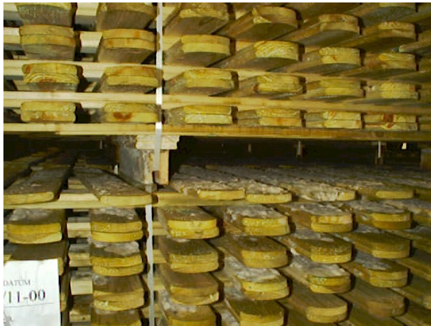
Figure 6. Characteristic attack by mould on the surface of wood treated with an arsenic and chromium free wood preservative.
