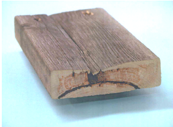
Figure 10. Severe decay in decking after approximately 8 years' in service.
