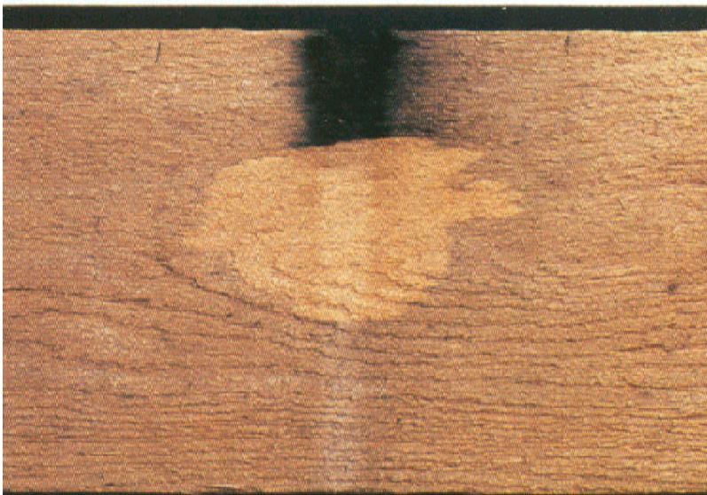
Photo 8. Iron stain bleached with Oxalic acid
