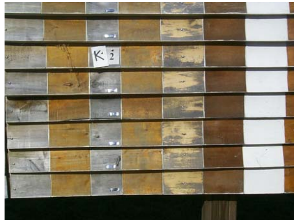
Figure 11: Section of test fence after 18 months exposure in Mississippi
