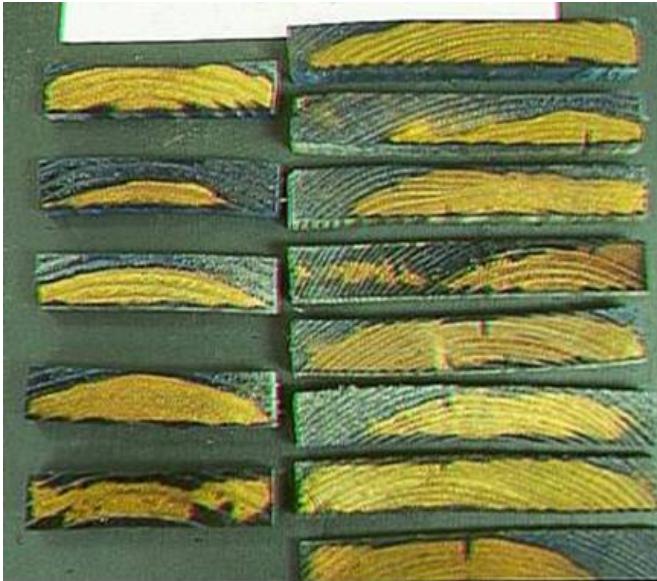
Photo 1: Scots pine treated with copper HDO
