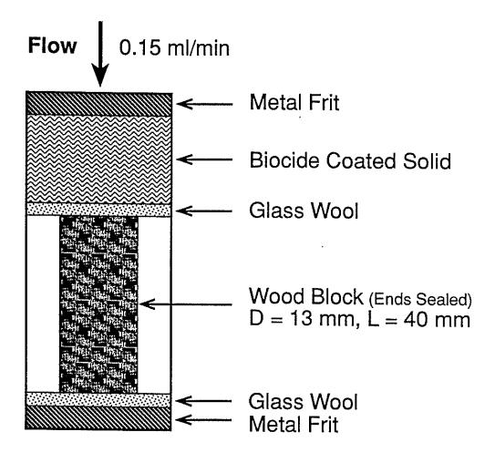
Figure 3. Vessel configuration employed for treatment of Douglas-fir dowels with selected biocides solubilized in supercritical fluids.
