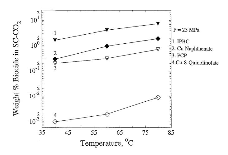
Figure 1. Solubility levels of biocides in supercritical carbon dioxide at 250 Bar and 40,60, or 80°C.
