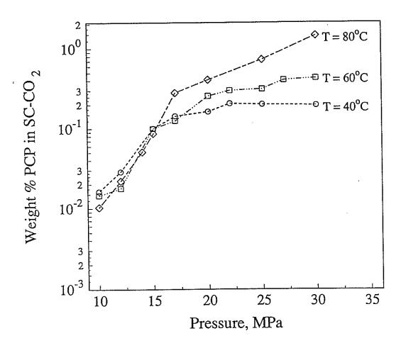
Figure 2. Solubility of pentachlorophenol in supercritical carbon dioxide at selected temperatures and pressures.
