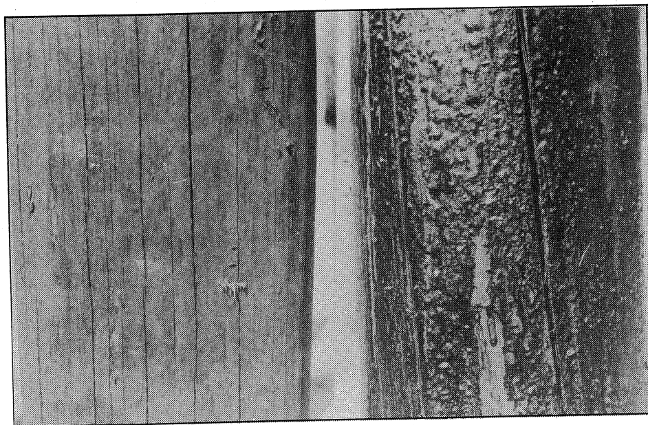
Figure 5. The Surface of Two Poles Treated with Creosote and Exposed for 6 Months in the Field. The Pole to the Left was Water Sprayed for 2 Months Immediately After Debarking and Then Dried. The Pole to the Right was Dried Immediately After Barking
