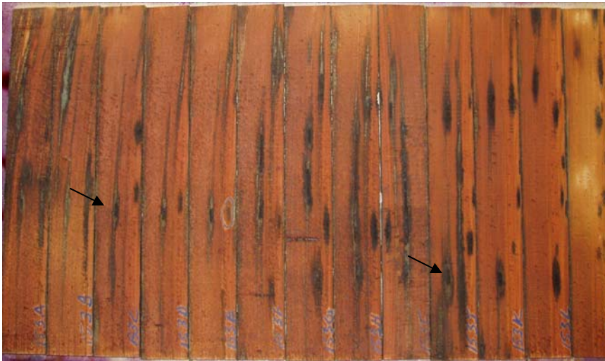
Figure 2. Example of ACQ penetration in western redcedar with T. blondeli galleries. The black color was caused by a reaction between Chrome Azurol S and the copper component of ACQ indicating that a majority of the galleries were penetrated by the preservative. Note that, the chemical did not diffuse away from the galleries.
