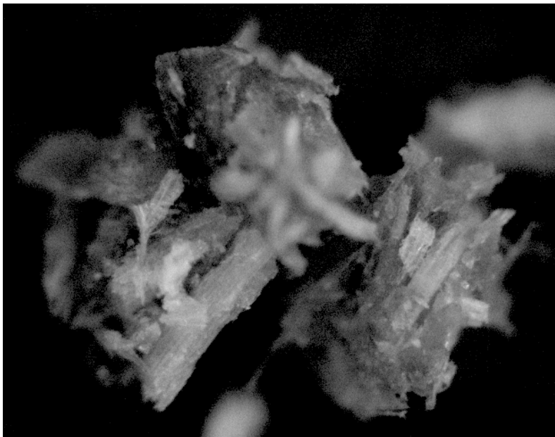
Figure 7. Micrograph (6x) of frass produced by a larva in contact with a 4mm thick ponderosa pine untreated veneer barrier with rounded edges on the individual particles suggestive of digestion of the wood.
