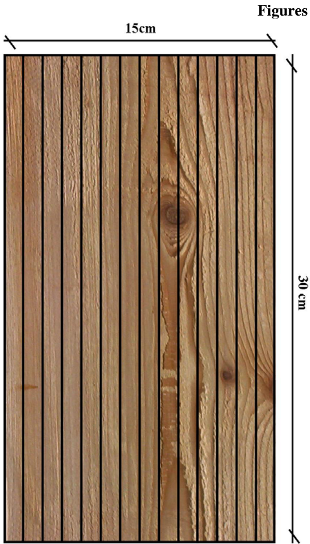
Figure 1. Cutting diagram for the penetration samples showing the widest face of the treated cedar block and the location of the cuts to produce 10mm thick strips. The dissection of the samples in this manner allowed for the assessment of preservative penetration into the insect galleries through the thickness of the sample.
