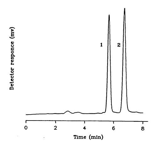
Figure 1.- Calibration standard 1-DoDAB (200  $\mu$ g/ml), 2-DDAC (200  $\mu$ g/ml)
