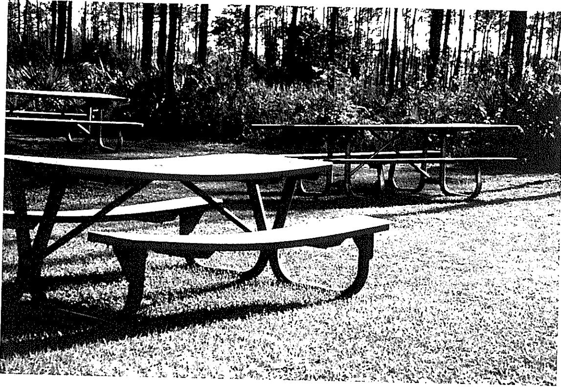
Figure 1 Sagging recycled-plastic-lumber picnic table. The level tables in the background are pressure-treated wood.
