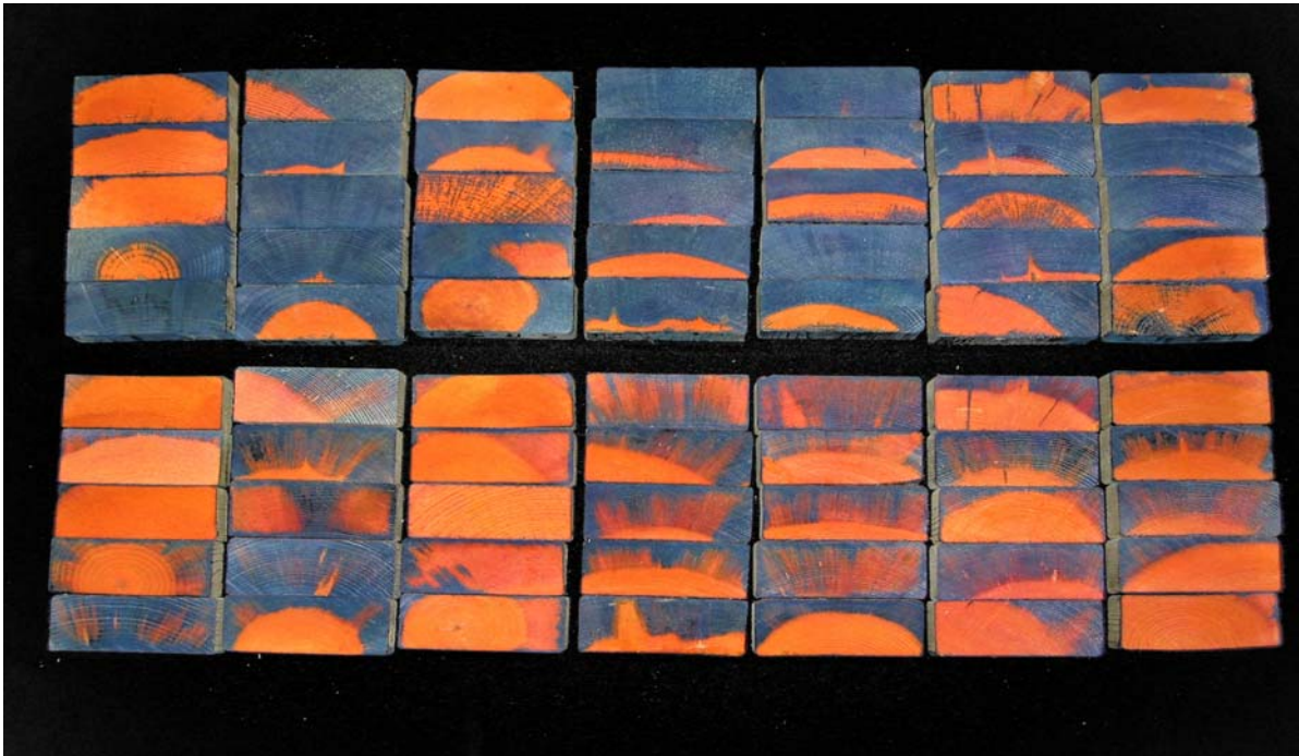
Figure 5: Non-stained Specimens – Pressure (top) vs. Dip Treated (24 hours soak)
