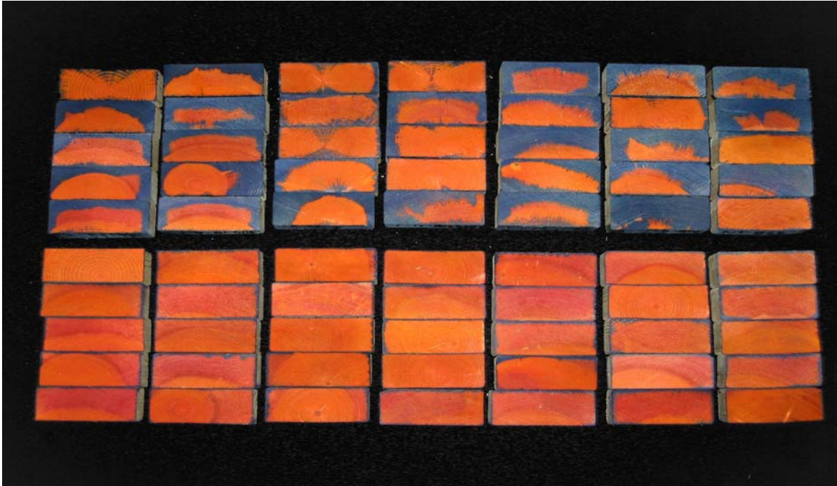
Figure 5: Non-stained Specimens – Pressure (top) vs. Dip Treated (24 hours soak)
