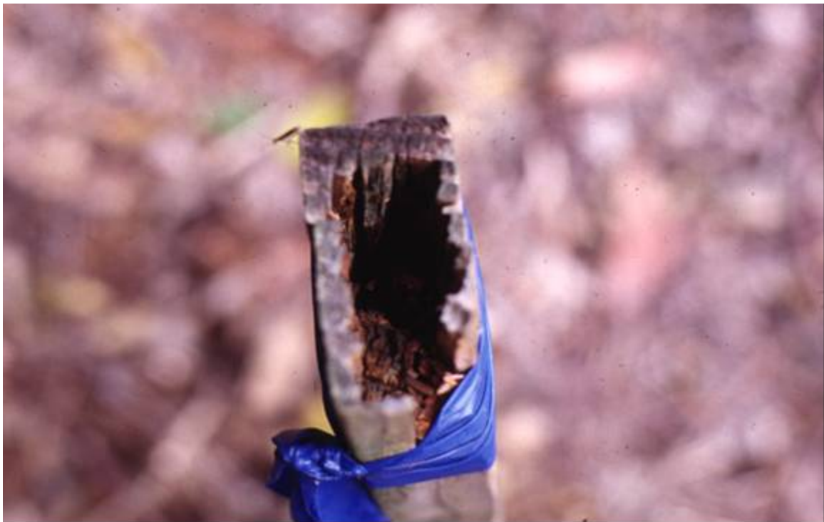
Figure 4. Shell Treatment Susceptibility to the FST. Sample of CCA-treated Douglas-fir exposed to the FST in Hilo, HI for one year in a covered, above-ground test.
