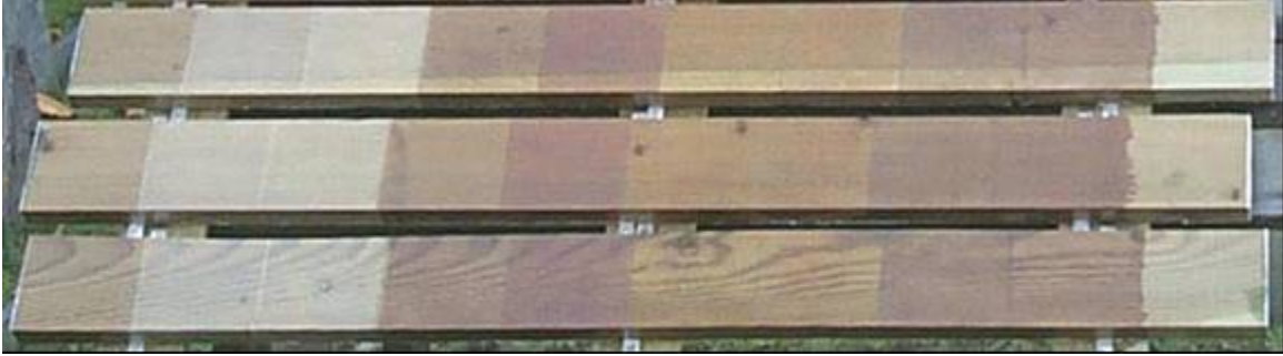
Figure 1: Example of siding immediately after installation, CCA-treated. F1 to F9 and control from left to right.)
