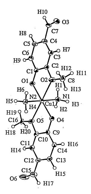
Fig. 1. Perspective view of Cu(II)-bis(vanillinato)bis(ammonia) with the atomic numbering; 33% probability thermal ellipsods are shown for the non-hydrogen atoms.
