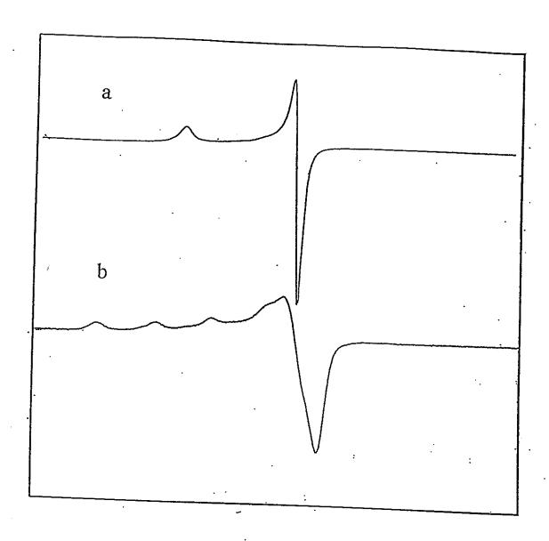
Fig. 3. ESR spectra of vanillin-copper complex a) solid at room temperature. b) in DMSO solution at 115 K.
