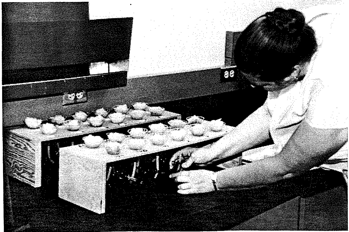
Figure 6 Baermann funnels containing wood shavings wrapped in Kimwipes and covered with water. Nematodes in solution obtained by opening pinchcock clamp on rubber tube.
