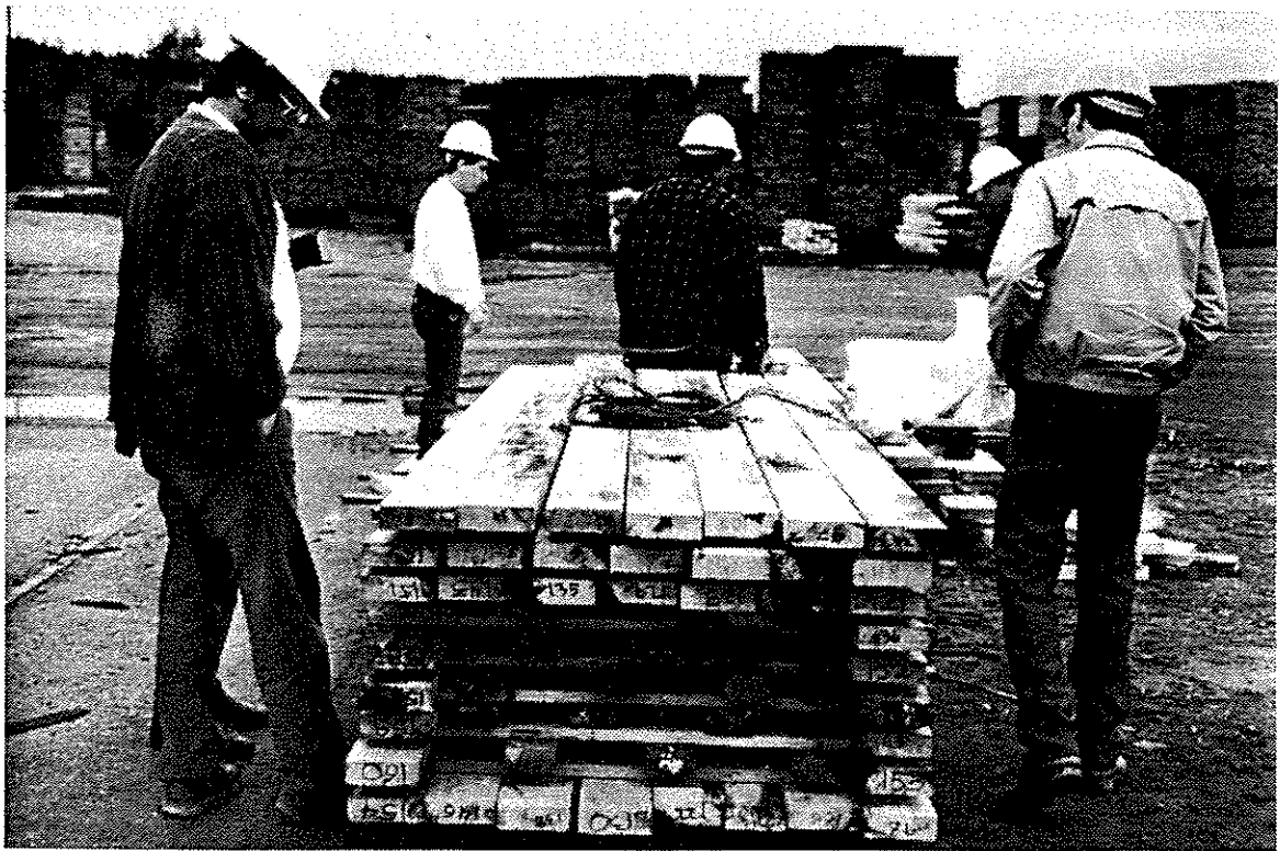
Figure 11 Experimental package of sapstained and PWN infested, ponderosa pine (dark boards), surrounded by Monochamus infested boards of white pine (light boards), all wired with thermocouples, at dehumidification kiln of Ashley Colter Ltd.
