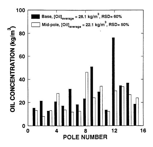
Figure 15. Oil concentration in fifteen 1983 in-service poles at two longitudinal positions
