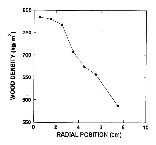
Figure 6. Variation of wood density along the radius of the pole
