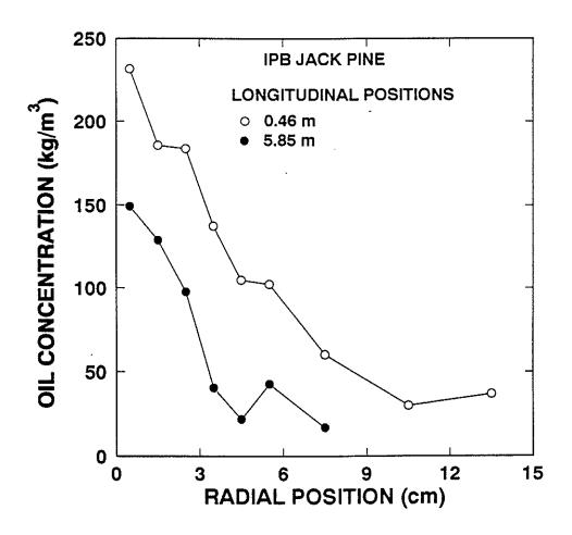
Figure 11. Oil radial distribution at two longitudinal positions
