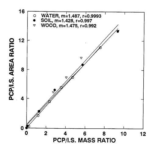
Figure 2. PCP calibration curves obtained by different preparation modes
