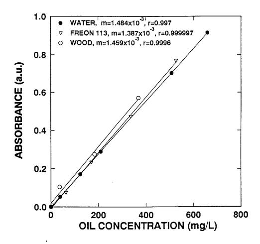
Figure 3. Oil calibration curves obtained by different preparation modes
