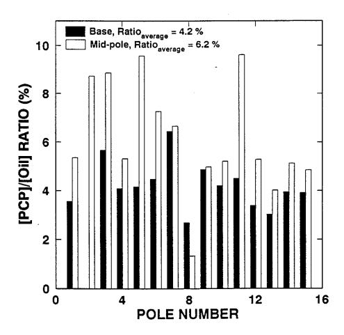
Figure 16. [PCP]/[Oil] ratio in fifteen 1983 in-service poles at two longitudinal positions
