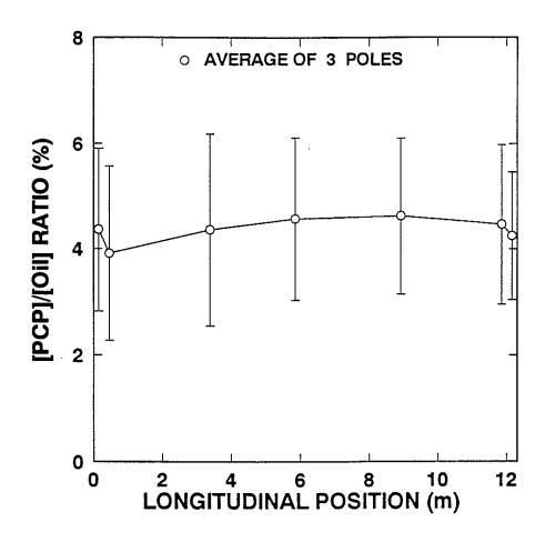
Figure 17. Longitudinal distribution of [PCP]/[Oil] ratio in 1990 freshly treated IPB poles
