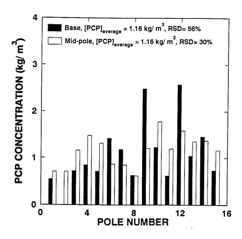
Figure 14. PCP concentration in fifteen 1983 in-service poles at two longitudinal positions
