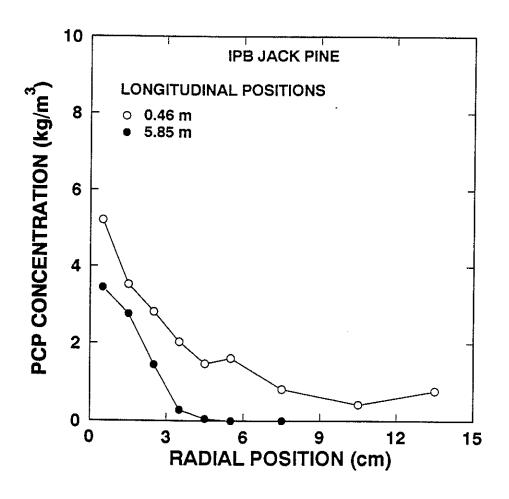
Figure 10. PCP radial distribution at two longitudinal positions
