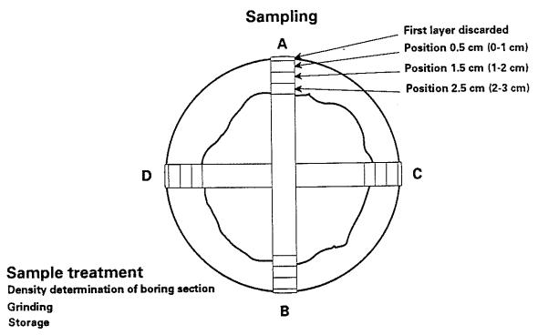
Figure 5. Wood sampling procedure for PCP and oil radial distribution in poles
