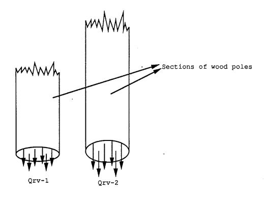
Figure 2. Schematic diagram showing loss of PCP in block1.
