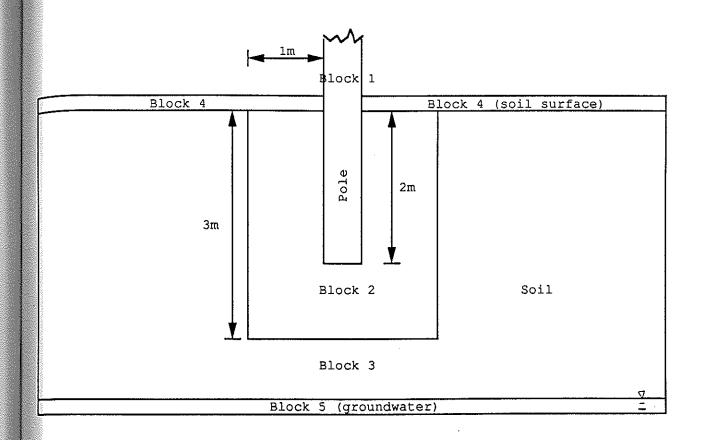
Figure 1. Schematic diagram showing the five blocks reflecting the PCP migration from treated poles.
