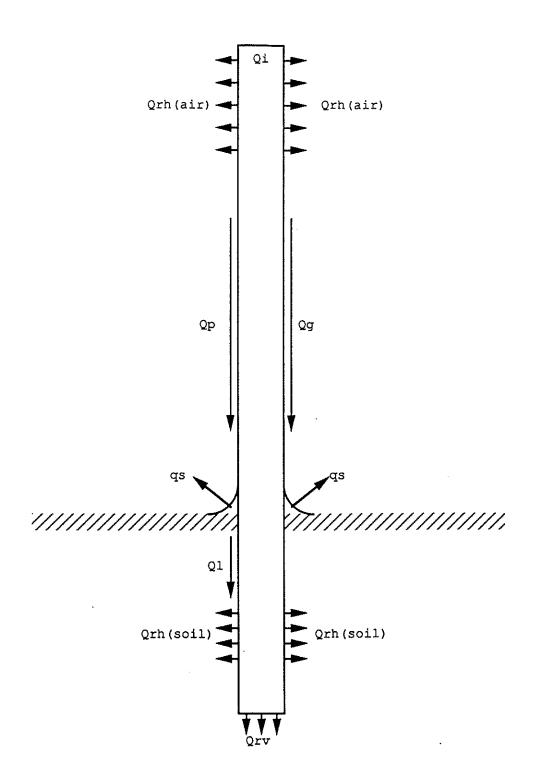
Figure 3. Schematic diagram showing the downward movement of pentachlorophenol in poles in service
