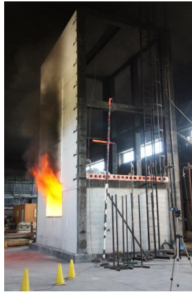
Figure 9 – CAN/ULC-S134 Exterior wall test (FPI/NRC/CWC Mid-rise consortium)
