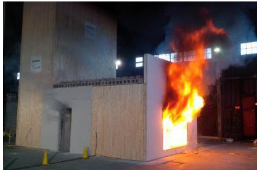
Figure 11 – Full-scale demonstration fire of exit shaft
