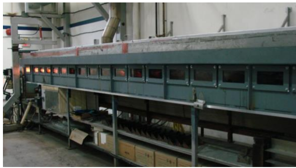
Figure 6 – CAN/ULC-S102 25-ft Steiner tunnel
