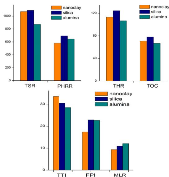
**Figure 5: Cone calorimeter most important parameters**
