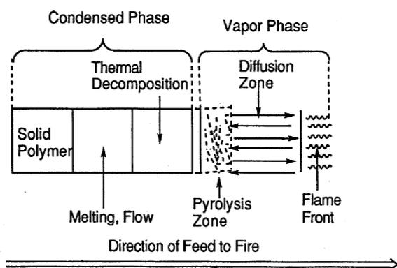
**Figure 2: representation of combustion phases (Stevens, 1999)**
