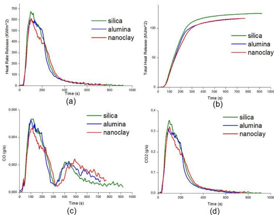
**Figure 4: Cone calorimeter results of 20WPC samples filled with 3% additives: (a) Heat Release Rate HRR (KW/m<sup>2</sup>), (b) Total Heat Release THR (MJ/m<sup>2</sup>), (c) CO production (g/s) and (d) CO<sub>2</sub> production (g/s).**
