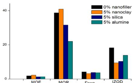
Figure 3: Mechanical test results for 40WHDPE nanofilled with 5%.
