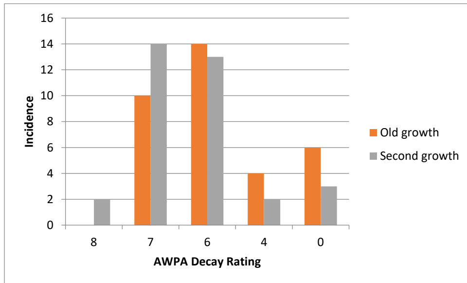
Figure 1: Distribution of decay ratings after 15 years for non-wrapped WRC posts
