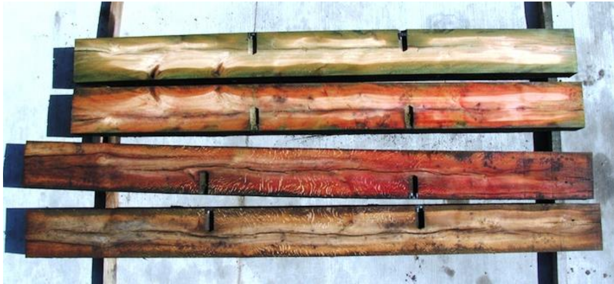
Fig. 1. Commercially dual treated borate (Cellutreat® liquid 50) and copper naphthenate (QNAP®) bridge timbers. Timbers have been rip sawn after borate and plug (BTX®) installation and Boulton treatment, and one half subsequently curcumin sprayed (Smith and Williams 1969) to show the presence of borate (red in two middle pieces).
