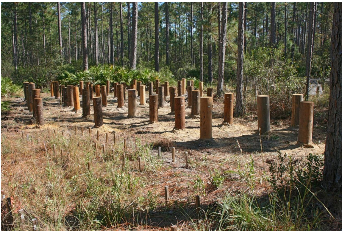
Figure 4. Pole stub testing of DCOI in southern pine, Gainesville FL
