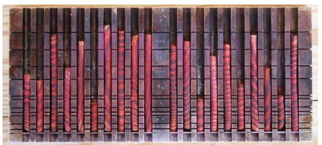
Charge 4: Southern Pine Crossarms (0/20 failures)
