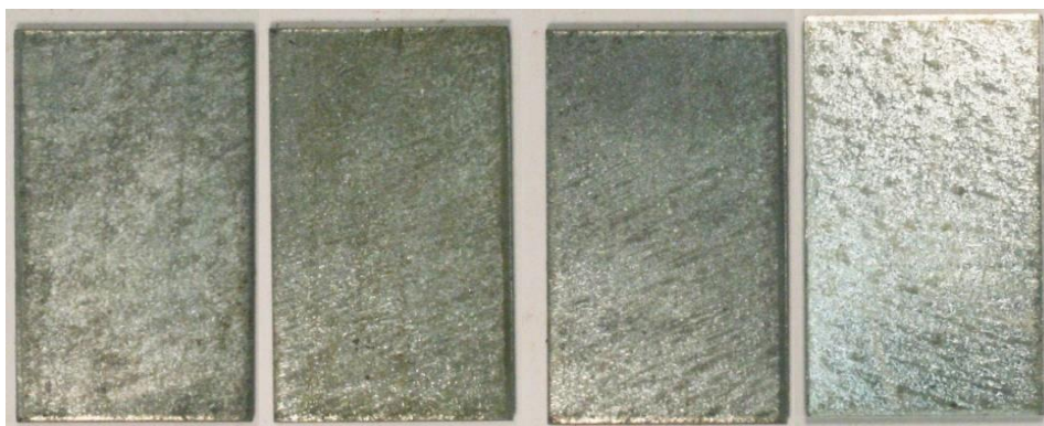
Figure 8A. Appearance of the G185 metal coupons before and after exposure for 408 hours in the AWP E12 corrosion procedure
