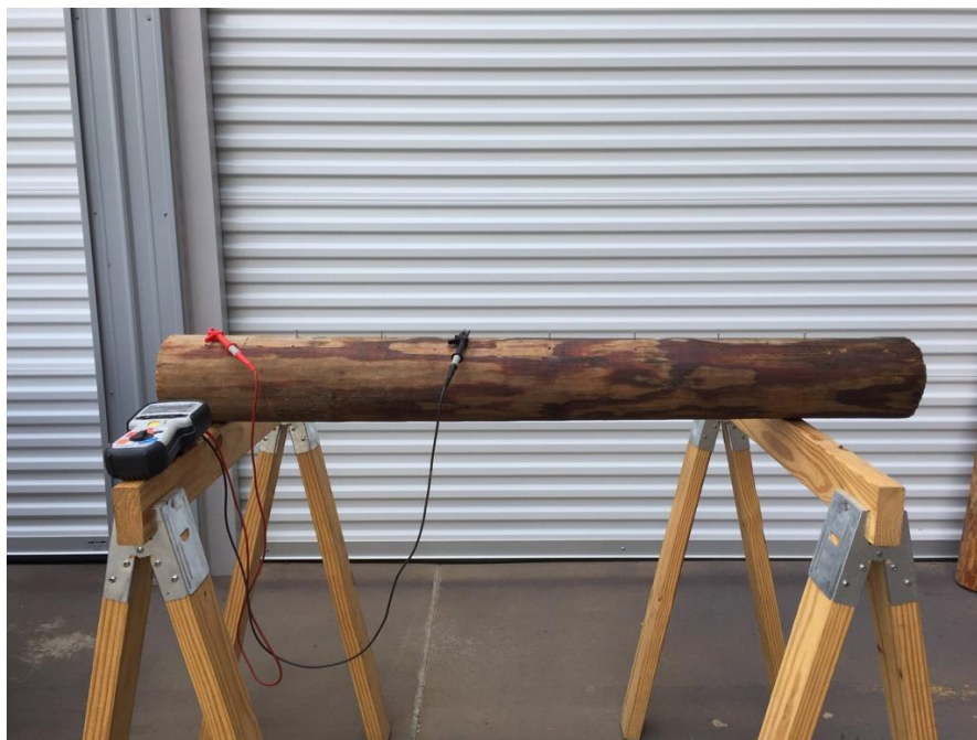
Figure 7 Test Setup for Resistance Measurements
