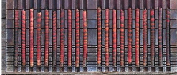
Charge 1: 20 Class 5 40' SYP Poles (0/20 failures)
