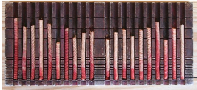
Charge 4: Douglas-fir Crossarms (1/20 failures)
