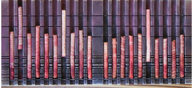
Charge 1: Douglas-fir Crossarms (3/20 failures)
