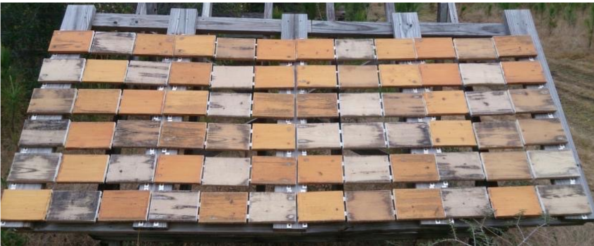
Figure 3: Samples after two years of exposure in Saucier, MS
