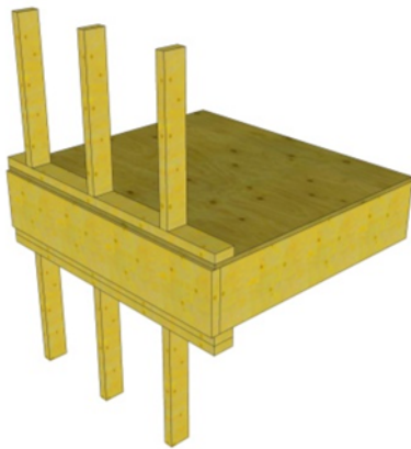
a. Platform framing
