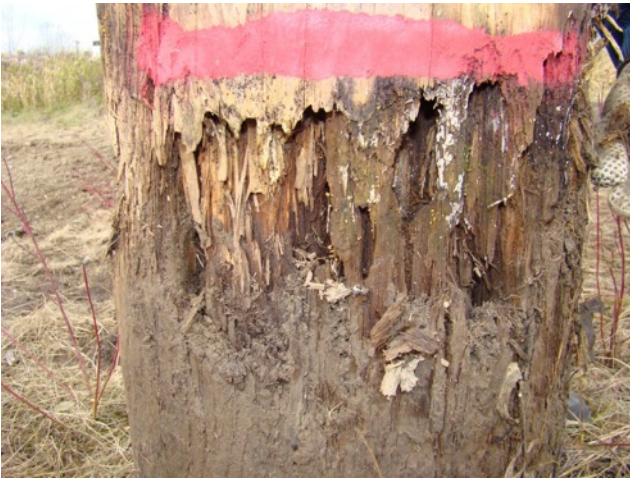
Figure 3: Ground line section for a red pine reference after 11 years in the ground
