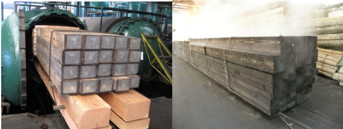
Figure 2. Hardwoods Cross-ties Before and After Treatment
