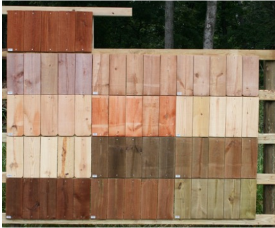
Photo 10: Vertical fence panel test in Harrisburg, NC illustrating a range of different colourant systems at the time installation.
