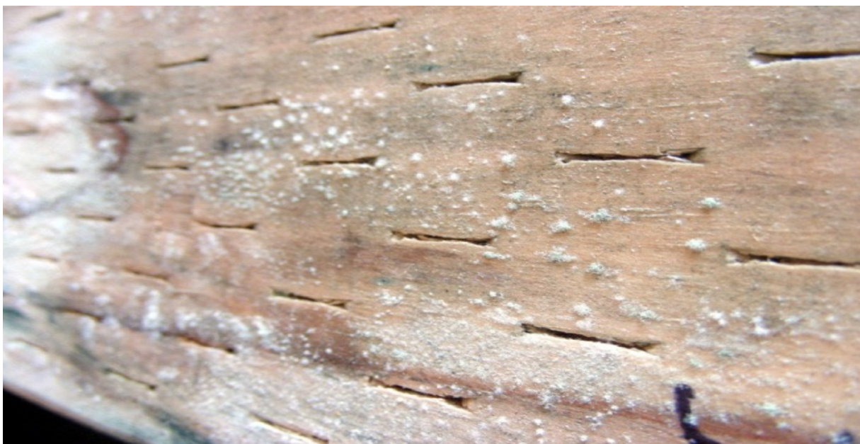
Figure 2. Example of unsightly mold on treated lumber (top). Example of Penicillium (bottom, left) and Trichoderma (bottom, right) genus at microscopic levels.
