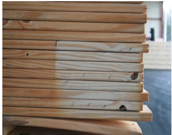
Photo 7: Colour variation in untreated southern pine associated with "sun burn". The light coloured corner was protected from exposure to the sun by a plastic placard.
