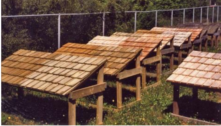
Figure 1 Pine, spruce and aspen shake test immediately after installation at Vancouver
