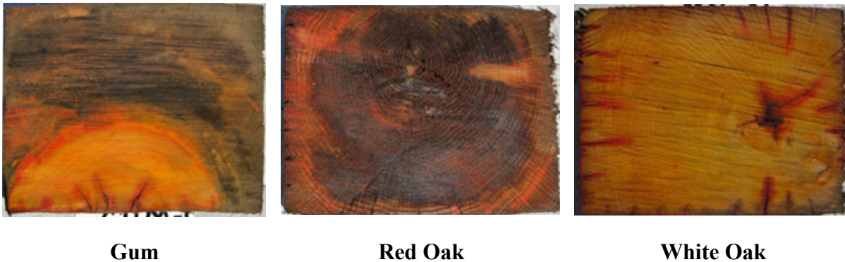
Figure 4. Tie Cross Sections with Borate Indicator
