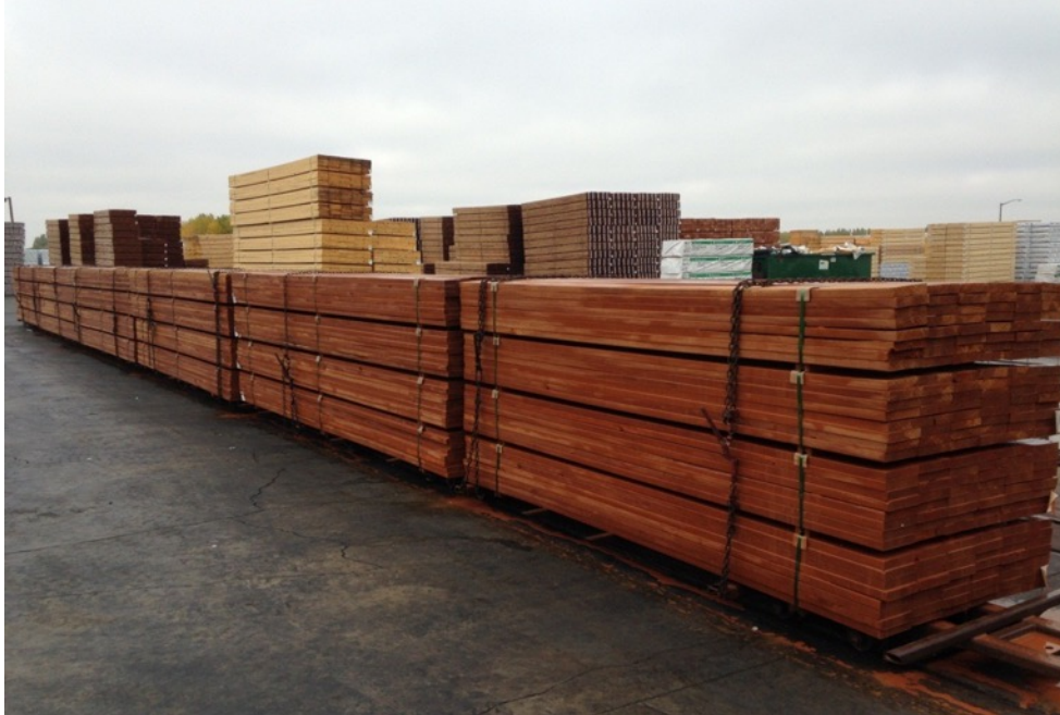
Figure 5. Southern yellow pine treated with micronized pigments plus a non-metallic preservative
