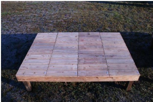
Photo 6: Colour variation in southern pine pressure treated with a pigment system. Column 1 from left Modified full cell cycle, Column 2 Short press time, Column 3 extended press time and Column 4 full cell cycle
