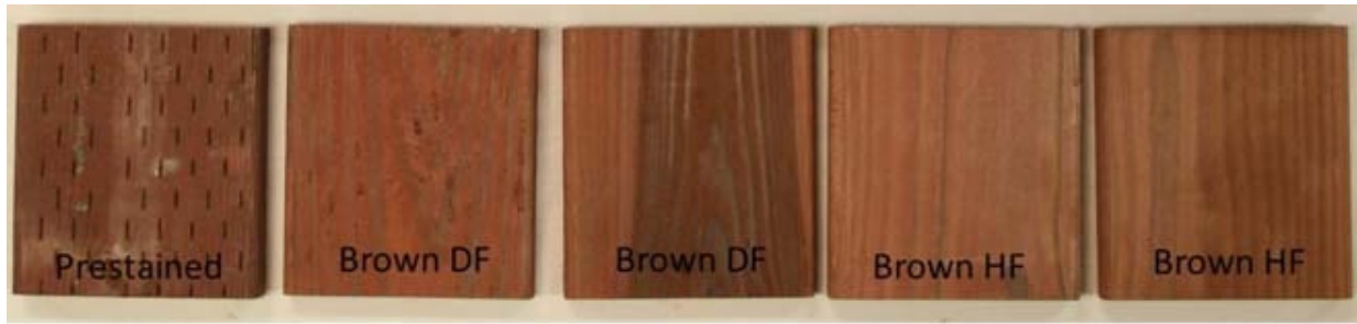
Photo 5: Colour variations with wood treated with a brown pigment dye system associated with heartwood/sapwood and species differences
