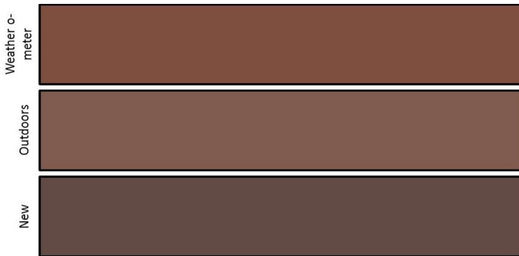
Photo 20: Preliminary results showing relative L* a* b* colour representation of matched samples of wood pressure treated with a colourant before exposure, after exposure outdoors and after exposure in an accelerated weather-o-meter.
