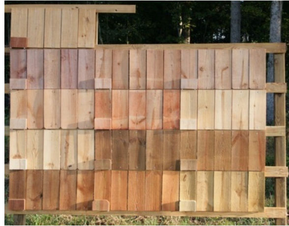
Photo 11: The same fence panel test after 43 weeks exposure. The small samples in the bottom left corner of each group are unexposed retains to illustrate the change from the original colour. It can be readily observed that some changes are quite pronounced.
