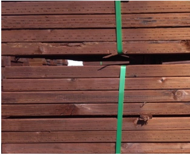
Photo 8: Colouration due to "sun burn" in lumber pressure treated with brown dye/ pigment formulation
