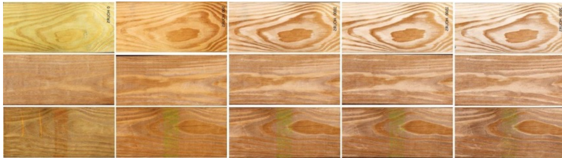
Photo 17: Accelerated Weather-o-meter exposure of southern pine pressure treated with a brown pigment colourant for different exposure times up to 2000 hours.
