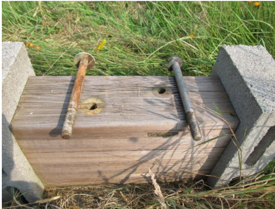
Figure 9 Rust on galvanized bolt in an ACQ-treated sample
