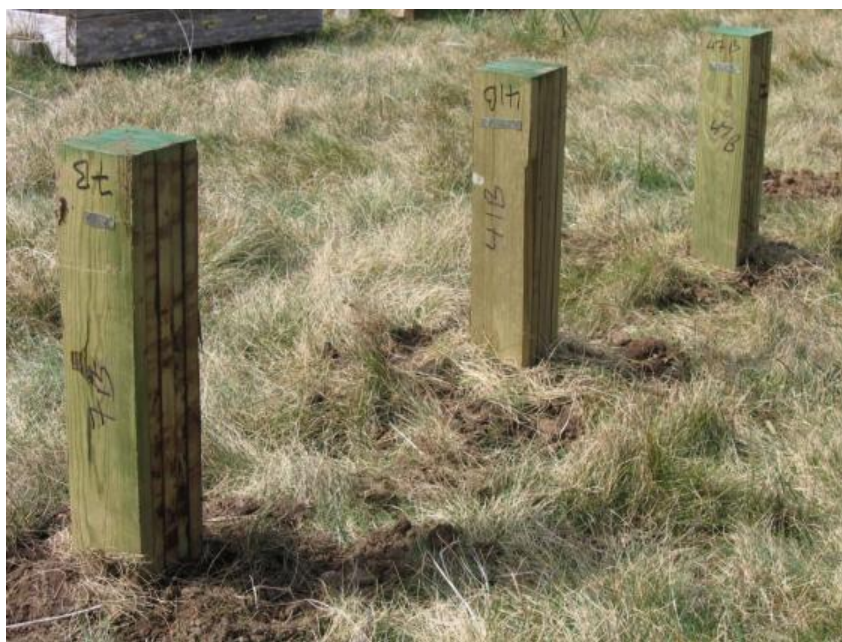
Figure 4 Glulam posts buried vertically to half depth in the ground
