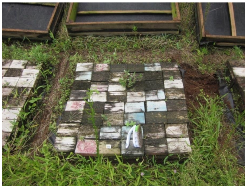
Figure 2. Example of an E18 Ground proximity decay test prior to the 18-month assessment after removal of vegetation showing heavy algal growth on the upper surfaces.
