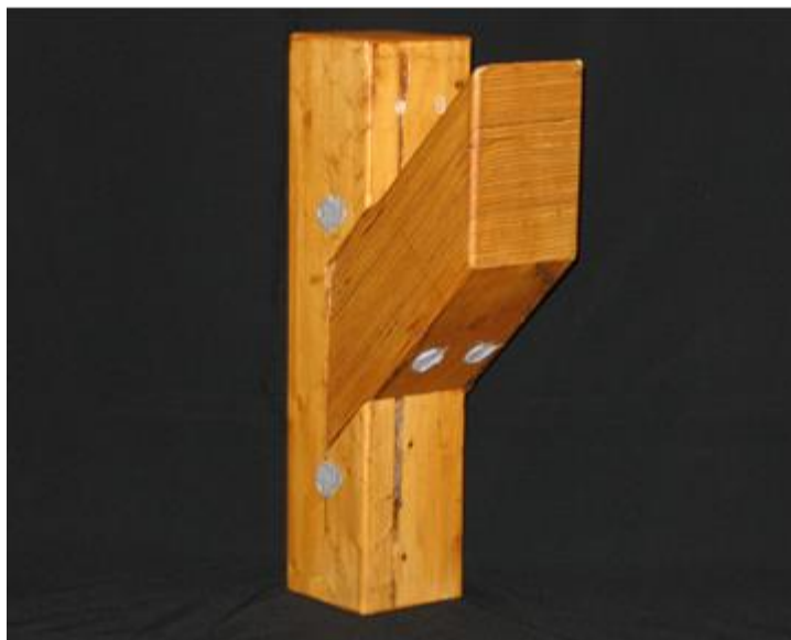
Figure 2 Borate/glycol-treated \gamma -joint showing copper/borate rod locations
