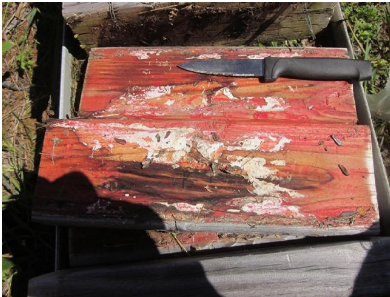
Figure 6. Example of the center sample of an Eco Red Shield I treated sample after 18 months of exposure in the sandwich test showing surface decay.
