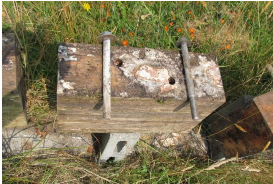
Figure 12 More extensive mycelial growth on the underside of an untreated Pacific silver fir glulam beam at the end with the stainless steel bolt.
