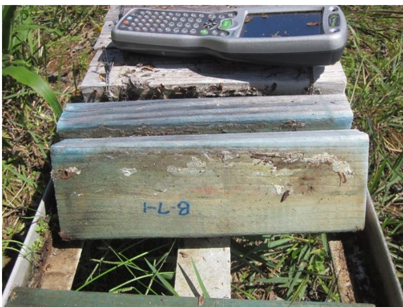
Figure 7. Example of the middle sample of a BluWood sandwich showing white fungal mycelium and slight surface decay after 18 months of exposure.
