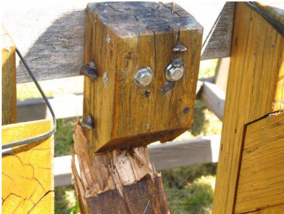
Figure 7 Failure of untreated black spruce glulam unit at six years of exposure
