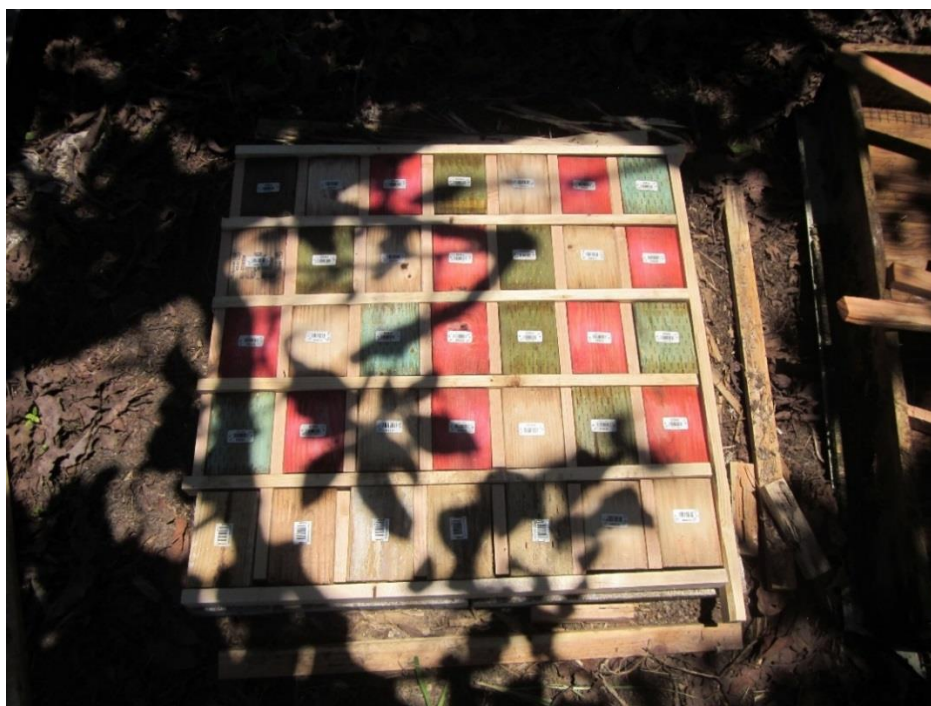
Figure 1. Example of a termite array with samples treated with Eco Red Shield II, HiBor or left untreated in the E26 Ground Proximity termite test after installation in June 2015.
