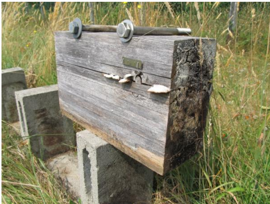
Figure 11 Fruitbodies of Gloeophyllum sepiarium towards the end of an untreated lodgepole pine beam with the stainless steel bolt
