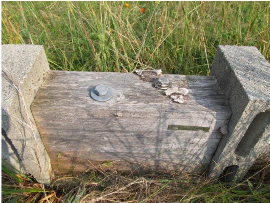
Figure 10 Fruitbodies of Gloeophyllum sepiarium on the top surface of an untreated Pacific silver fir glulam beam close to the stainless steel bolt.
