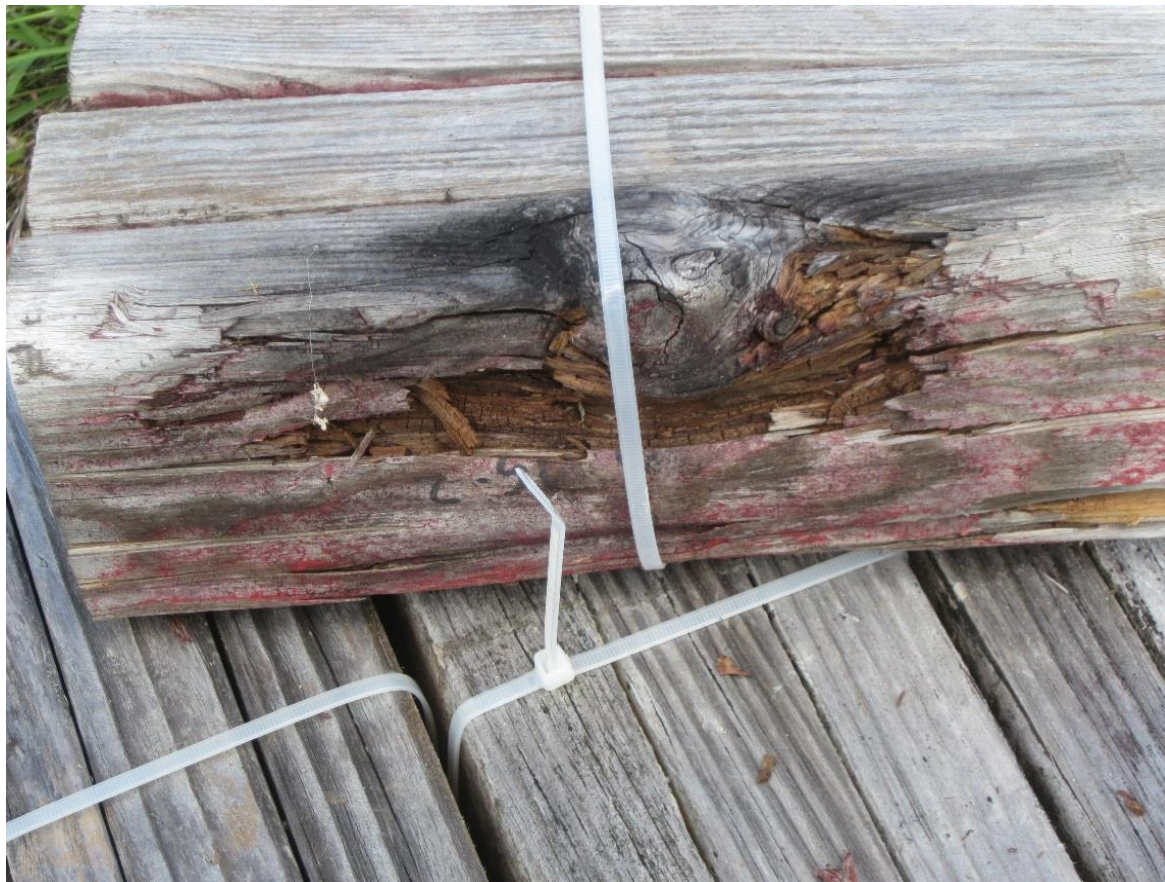
Figure 8. Example of an EcoRed Shield I sandwich showing advanced decay on the outside of the sandwich.
