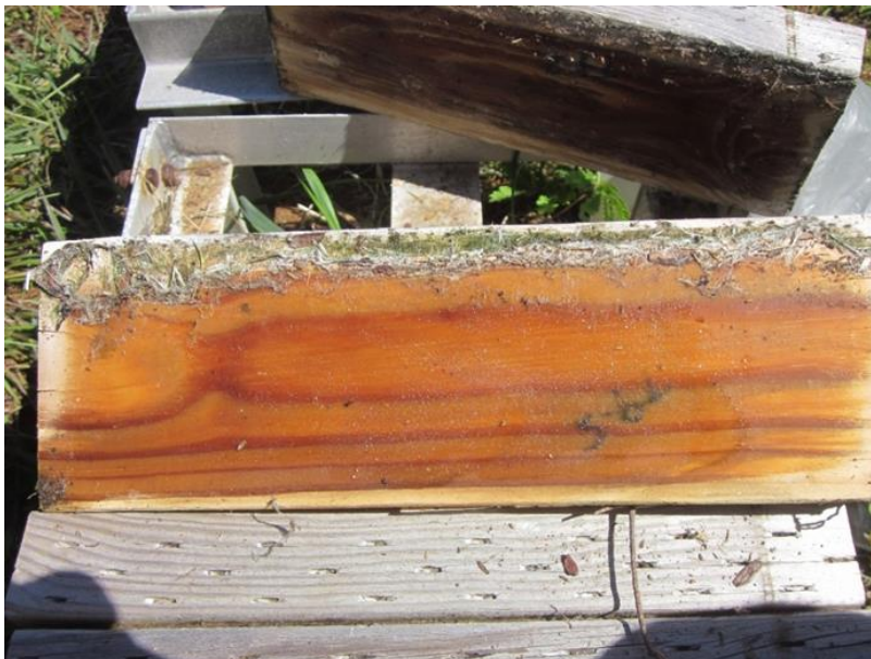
Figure 5. Example of a Timbersil treated sample from a sandwich test showing the collection of wood fibers on the upper, UV exposed surface.
