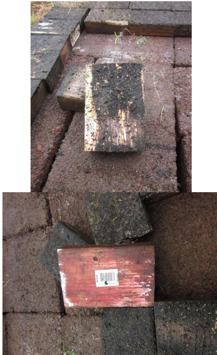
Figure 3. Examples of a non-treated control (left) showing extensive surface growth and slight decay and an Eco Red Shield I sample showing white fungal growth and decay.
