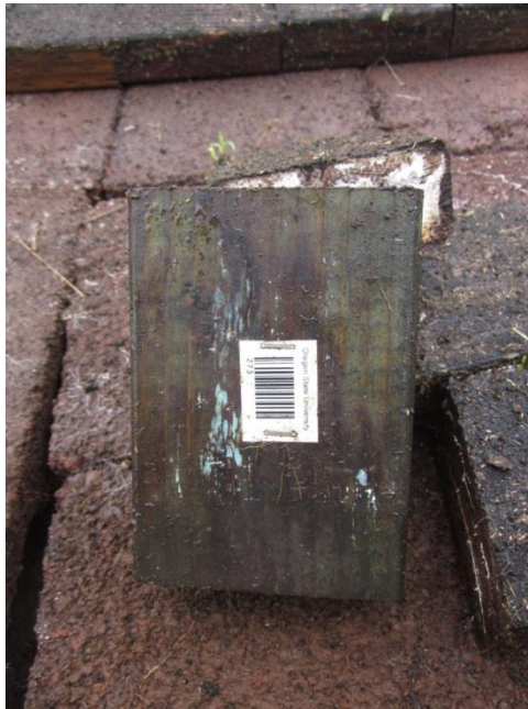
Figure 4. Example of a BluWood ground proximity sample after 24 months of exposure showing decay pockets with concentrations of the original blue dye used to color the wood.
