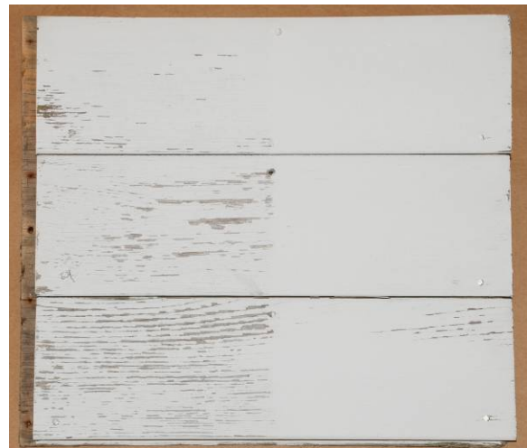
Figure 7. Western redcedar boards painted with oil-alkyd primer and one acrylic latex top-coat (left) and two top-coats (right) after 29 years outdoor exposure at the Forest Products Laboratory test site near Madison, Wisconsin
