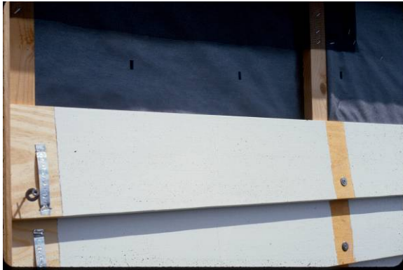
Figure 9. Boards on test fence showing rain screen on the left and no rain screen on the right
