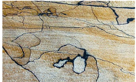
Fig.1 Pattern of zone lines and coloration characteristic to spalted wood
