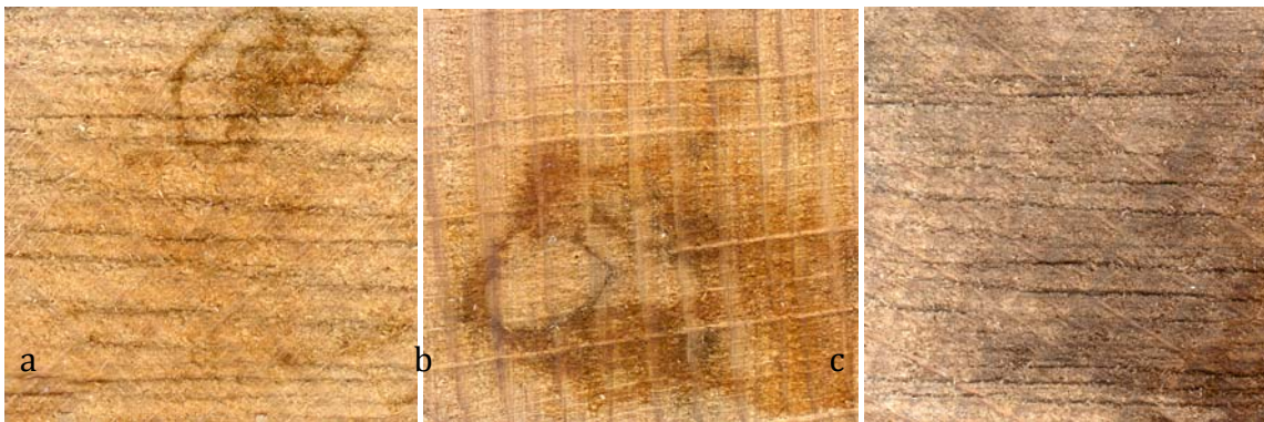
Fig.13 Representative samples of pigmentation produced by Inonotus hispidus in beech: a-control samples; b- beech with 7ppm catechol; c-beech with 700ppm catechol.
