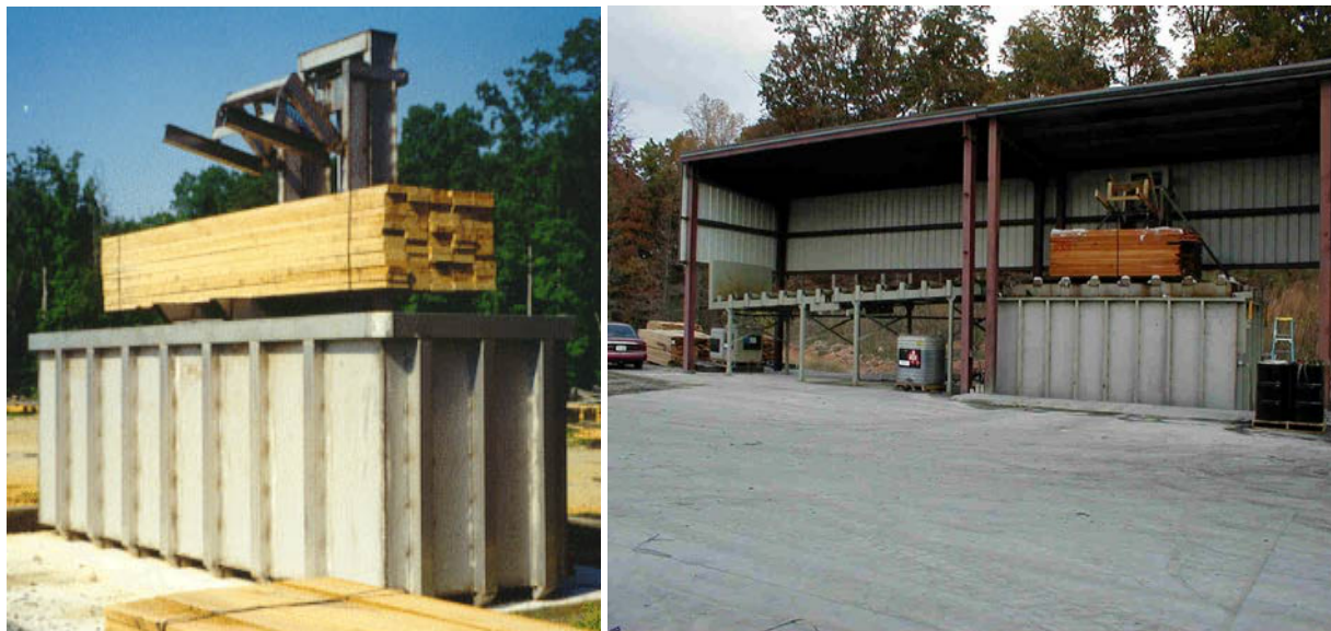
Figure 5. Dip Tank antisapstain treatment systems. Unit Dip Tank (left) and Unit Dip Tank with primary drip area.
