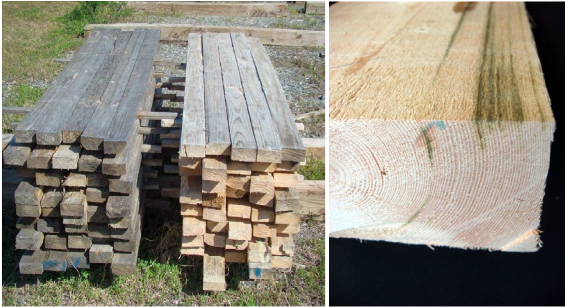
Figure 4. Examples of Non-microbial discolorations: Photochemical (top, left), Enzymatic (top, right), Chemical (middle) and Brownstain (bottom).
