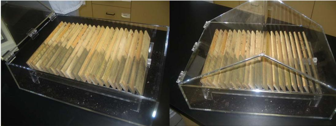
Figure 2. Mold boxes showing mold test specimens at the end of test.
