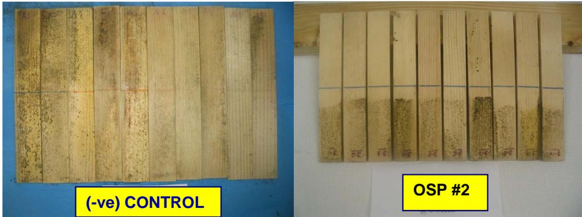
Figure 4. Mold specimens at the end of mold test.
