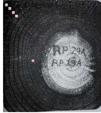
Figure 1. Drilling sample of treated red pine section (left) cut from a treated “4 x 4” (right).
