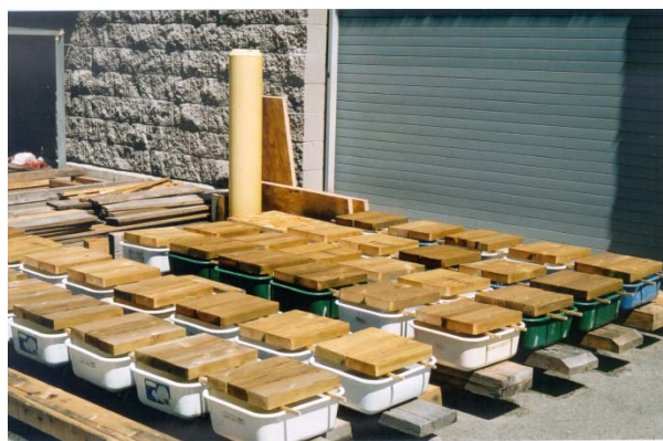
Figure 4 test samples exposed for measuring preservative mobility
