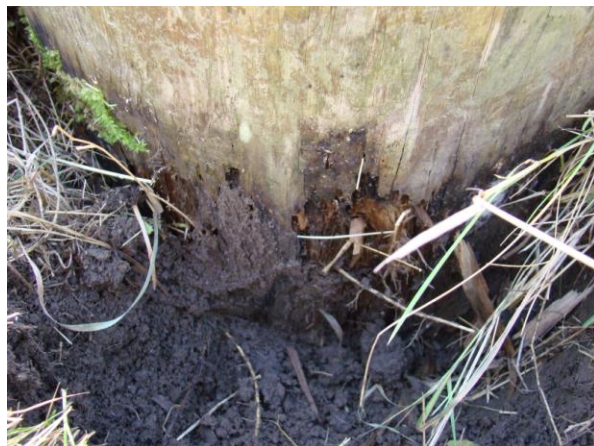
Figure 7: Degradation at the ground level for a reference section
