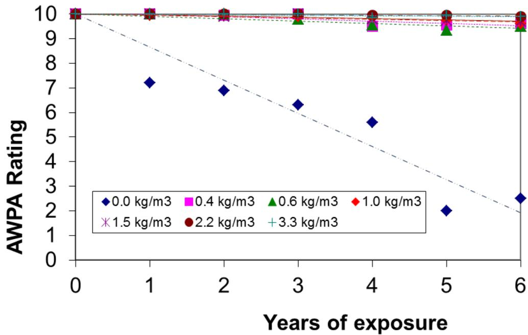
Figure 6 Performance (decay) of CA-B-treated white spruce stakes at Maple Ridge
