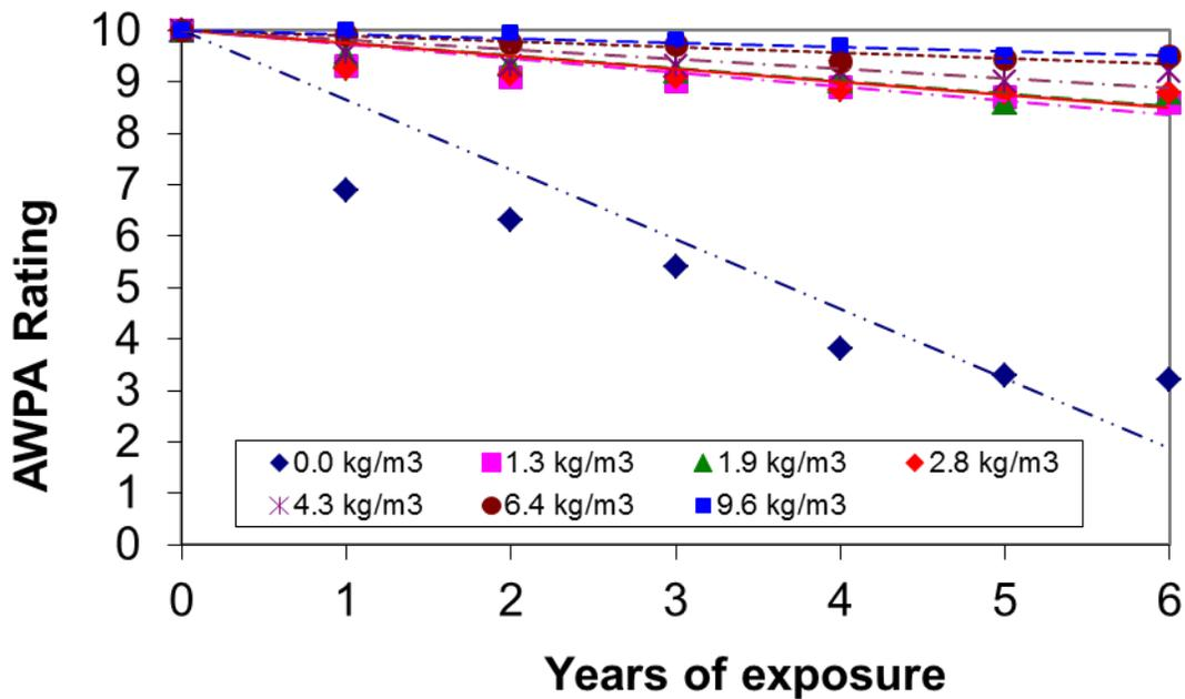
**Figure 8** Performance of ACQ-D-treated Pacific silver fir stakes at Maple Ridge
