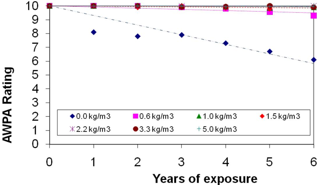
**Figure 4** Performance (decay) of CA-B-treated jack pine stakes at Maple Ridge
