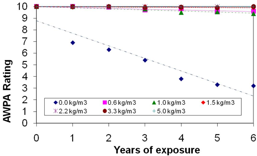
Figure 2 Performance (decay) of CA-B-treated Pacific silver fir stakes at Maple Ridge
