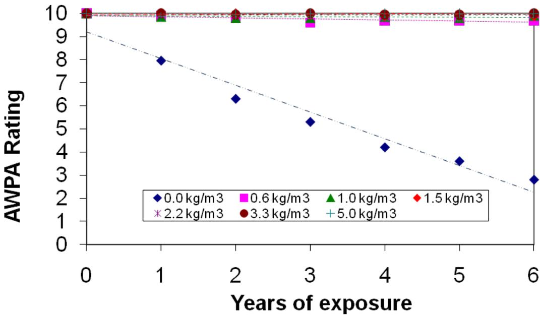
Figure 3 Performance (combined decay/termite) of CA-B-treated Pacific silver fir stakes at Kincardine
