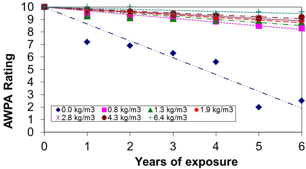
Figure 10 Performance of ACQ-D-treated white spruce stakes at Maple Ridge
