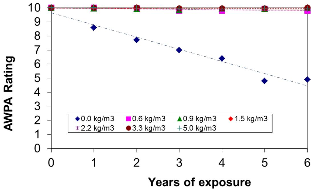
Figure 5 Performance (combined decay/termite) of CA-B-treated jack pine stakes at Kincardine
