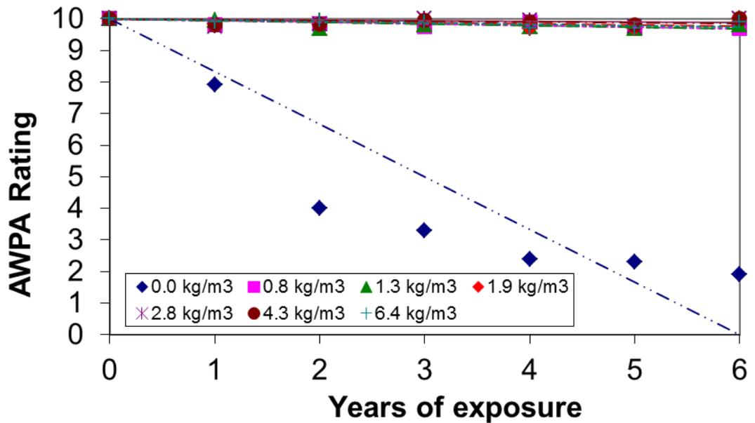
Figure 11 Performance (combined decay/termite) of ACQ-D-treated white spruce stakes at Kincardine
