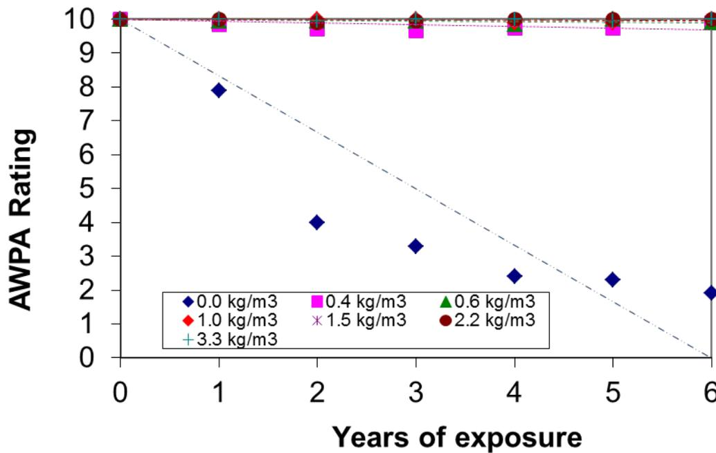
Figure 7 Performance (combined decay/termite) of CA-B-treated white spruce stakes at Kincardine
