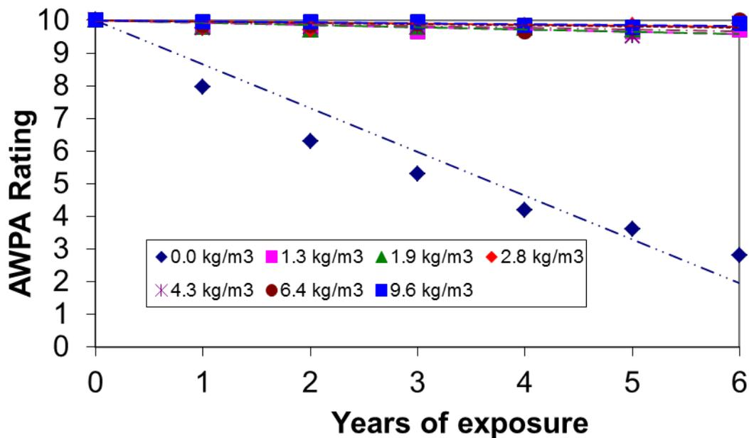
Figure 9 Performance (combined termite/decay) of ACQ-D-treated Pacific silver fir stakes at Kincardine
