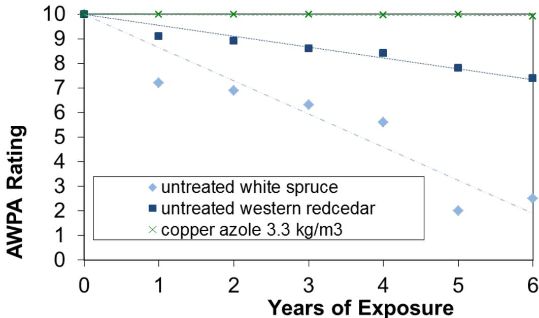
Figure 12 Performance of untreated western redcedar and spruce compared to CA-treated spruce
