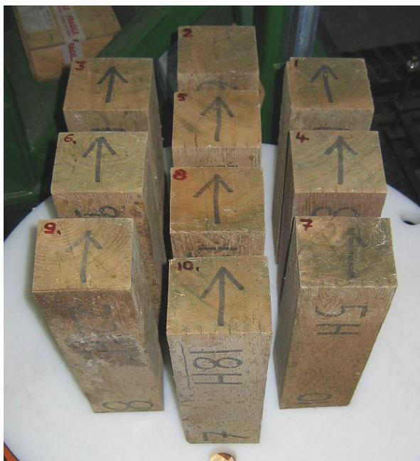
Figure 2 Dodai from Hawaii on CT scanner turntable
