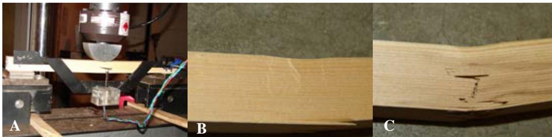
**Figure 5** *Bending strength test (A), compression failure (B) and tension failure (C)*
