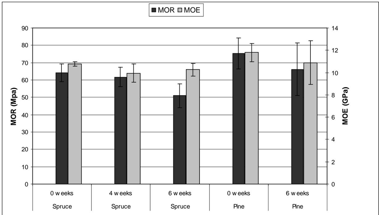
**Figure 4** *MOE and MOR results from the strength testing of spruce and pine samples biologically incised for with *D. squalens* versus control samples with no biological incising. Spruce sample size = eight; Pine sample size = 5. Error bars represent standard deviation.*
