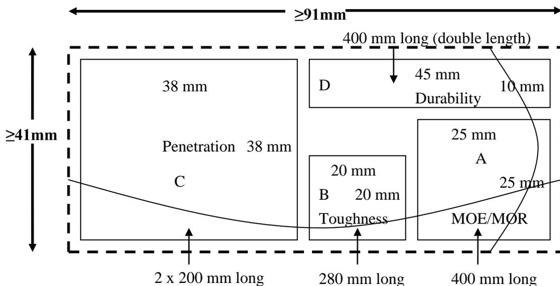
Figure 1 Cutting pattern for sub-samples from bio-incised 5 cm by 10 cm boards (cross section view).
