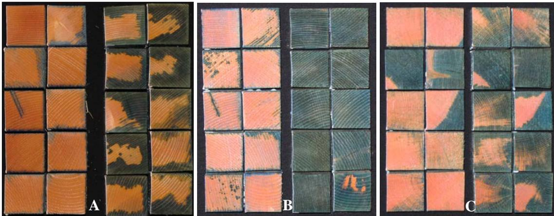
*Figure 2 ACQ uptake in 4 week exposed spruce (A), 6 week exposed spruce (B) and 6 week exposed pine (C) with controls (left) versus biologically-incised samples exposed to *D. squalens* (right). Blue coloration is from the copper indicator, chrome azurol S and represents the treated area*
