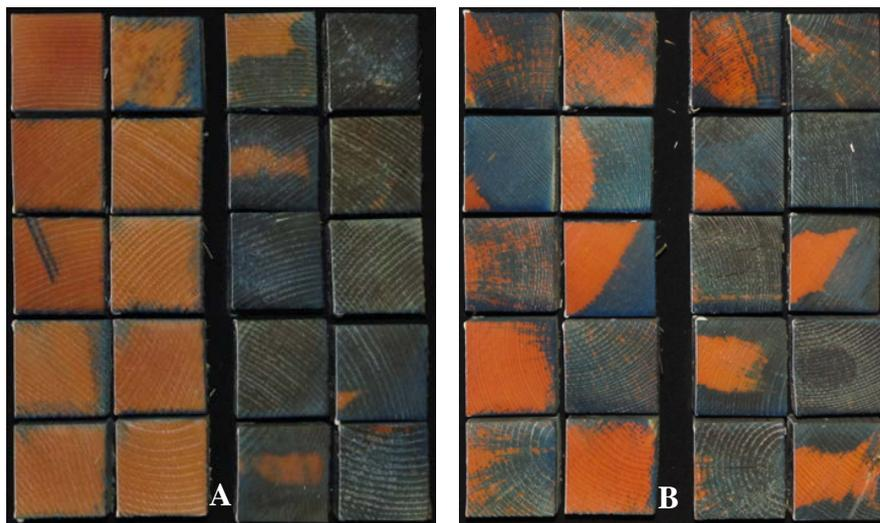
*Figure 3 MCA (0.9%) uptake in spruce (A) and pine (B) with controls (left) versus biologically-incised samples exposed to *D. squalens* for six weeks (right). Blue coloration is from the copper indicator, chrome azurol S and represents the treated area*
