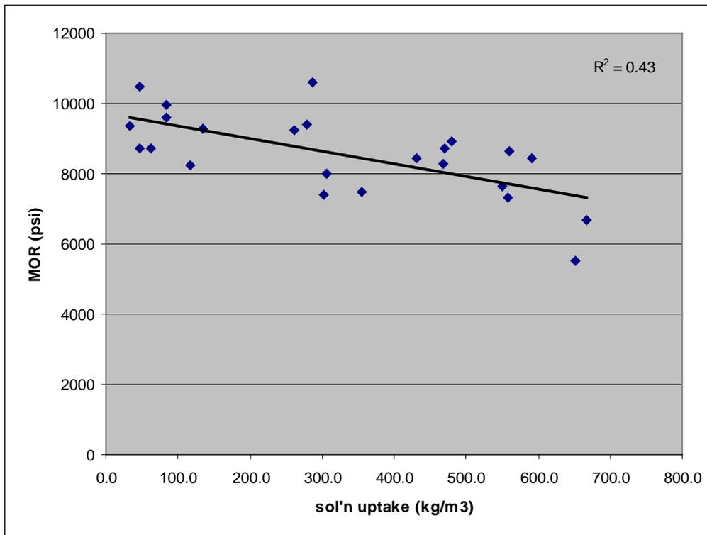
**Figure 6** Correlation between MOR and solution uptake for spruce samples including control, 4 week and 6 week biologically incised samples
