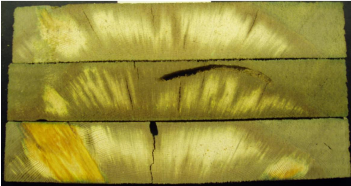
Figure 1. Example of copper penetration (green areas) in cross sections cut from unseasoned ponderosa pine containing active beetle infestations and pressure treated with ACQ.
