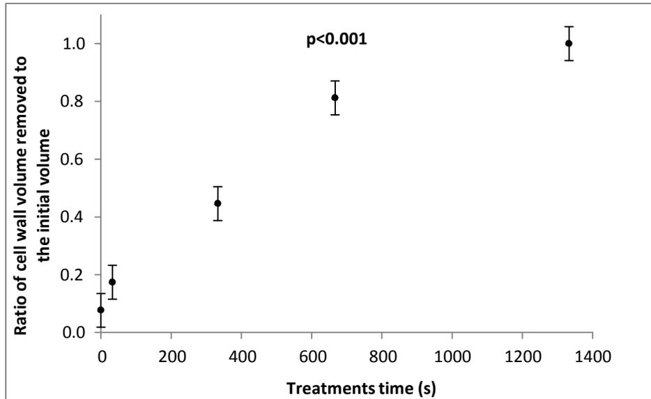
**Figure 6: Effect of plasma treatment time on the mass loss in yellow cedar and poplar specimens (results are averaged across species and cell walls [radial and tangential])**
