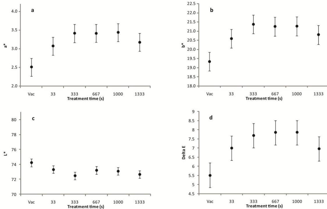
**Figure 11: Effect of the combination of plasma pretreatments of different durations with bleaching on the redness (a\*), yellowness (b\*), lightness (L\*) and total color change (delta E) of blue-stained lodgepole pine wood**
