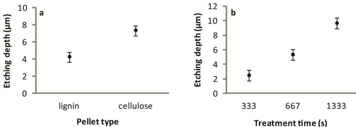
**Figure 7: Plasma etching of lignin and cellulose pellets (results averaged across plasma treatment time) (a), and treatment time (averaged across pellet type) (b) on the depth of etching of the pellets during plasma treatment**
