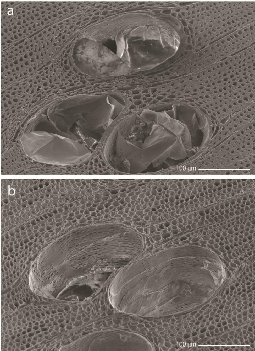
**Figure 4: SEM photomicrographs of transverse surface of rose gum (*E. grandis*): (a) untreated surface showing cross-cut fibers and three vessels occluded with tyloses and (b) surface subjected to plasma for 1333 s showing etching of fibers and removal of tyloses from two vessels**
