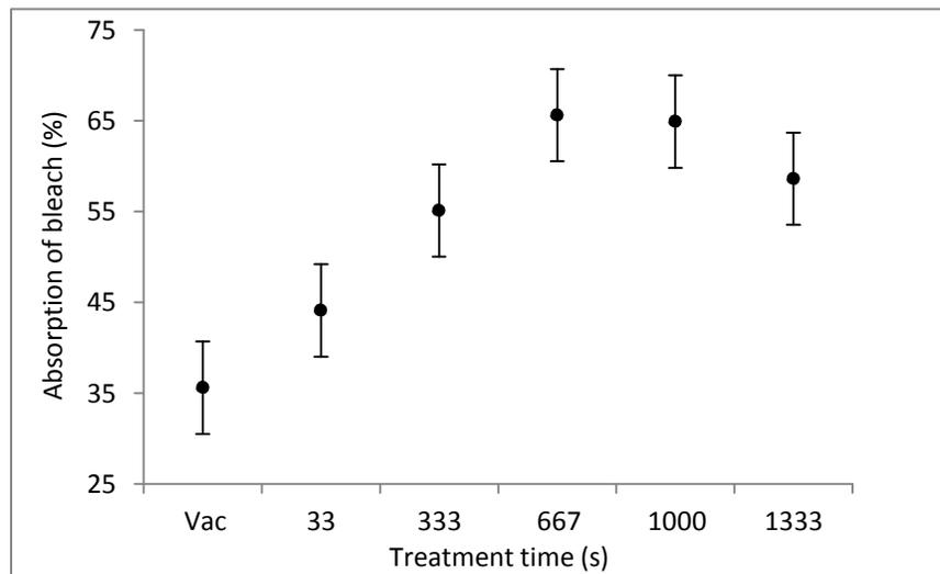
**Figure 10: Effect of plasma treatments on the absorption of bleach by blue-stained lodgepole pine wood**
