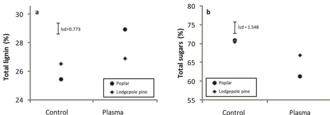
**Figure 8: Effect of plasma treatment (667 s) on lignin and sugar contents of thin veneers of lodgepole pine wood. Specimens exposed to vacuum acted as a control.**
