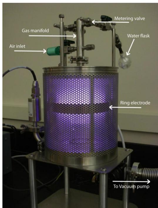
**Figure 1: Plasma reactor used to modify wood samples**
