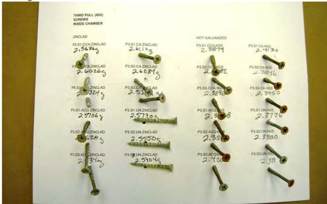
Figure 6. Visual Appearance of Fastener Specimens after 90 Days Exposure, Before Cleaning
