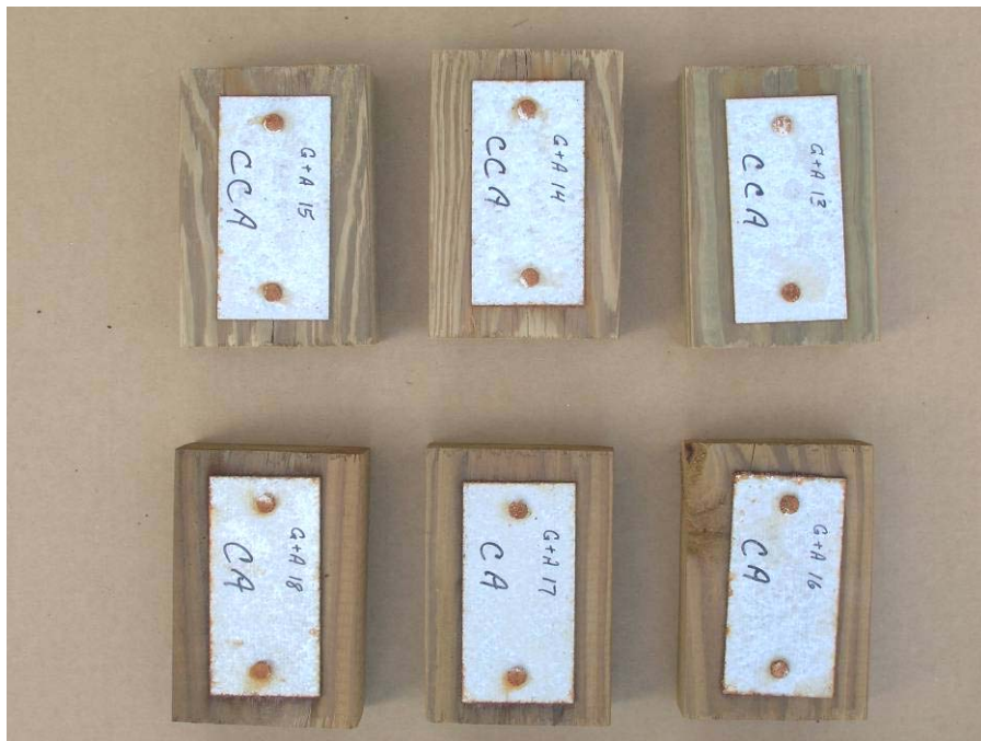
Figure 4. Visual Appearance of Sheet Steel Samples after 30 Days Exposure, Before Cleaning: CCA and CA Exposures
