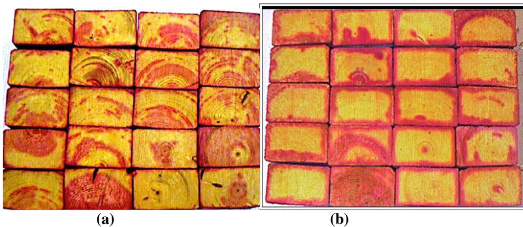
**Figure 4: Borate penetration in black spruce a) immediately after treatment; b) after 1 week diffusion period without drying**
