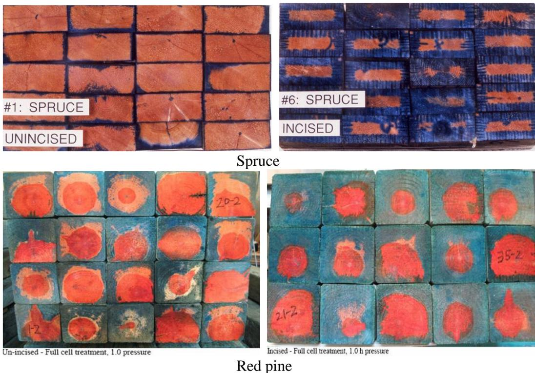
**Figure 6: Effect of incising on treatment of refractory spruce (top) and more permeable red pine (bottom)**
