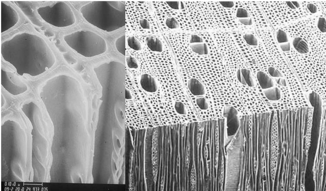
**Figure 1: Typical structure of a softwood (pine) and hardwood (birch) (SWST Slide set on Wood structure) Note the pine is much more highly magnified than the birch**
