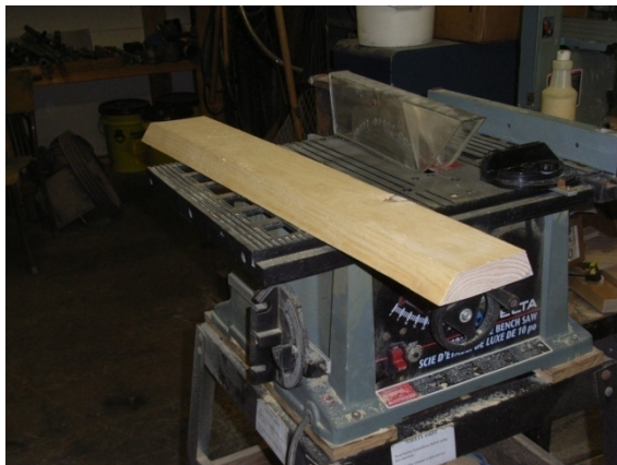
Fig. 4 Preparing kiln dried wood into planks
