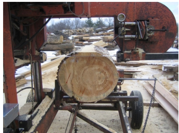
Fig. 3 Cutting flat sawn planks of sapwood
