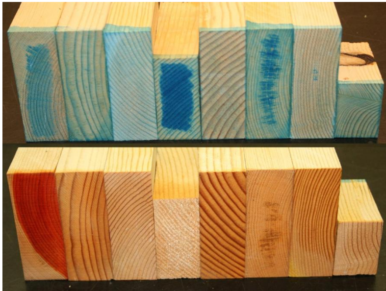
Photo 2: Freshly cut ends of millwork lumber treated with a clear non-metallic preservative system containing a water repellent additive before and after spraying with a blue dye. Untreated zones where the water repellent preservative has not penetrated are colored darker blue.
