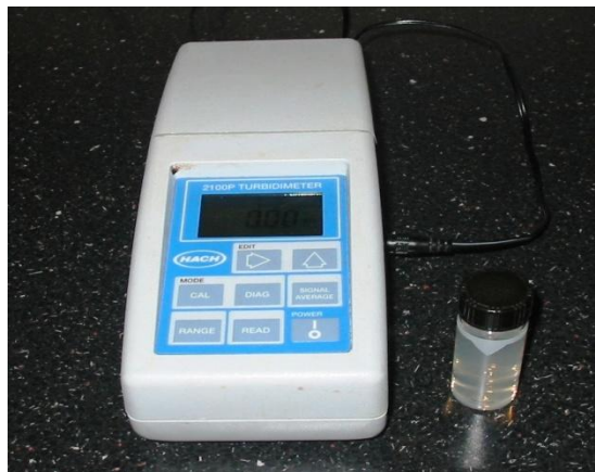
Photo 3: A simple and inexpensive turbidity meter for in-plant QC of water repellent stabilizers in solution.
