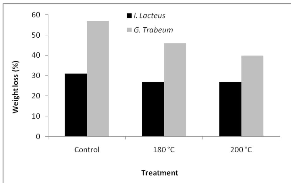
**Figure 5.** Weight loss for treated and control balsam fir wood samples after decay with exposure to white-rot fungus *Irpex lacteus* and brown-rot fungus *Gloeophyllum trabeum*
