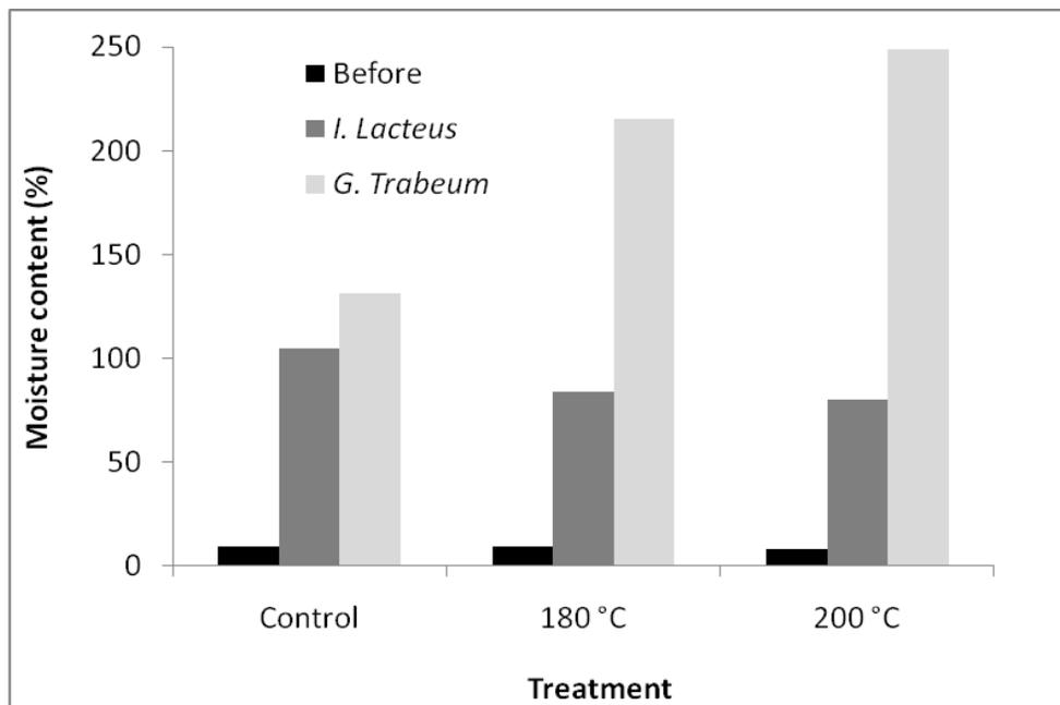
**Figure 4.** Moisture content of treated and control samples before and after decay with exposure to white-rot fungus *Irpex lacteus* and brown-rot fungus *Gloeophyllum trabeum*
