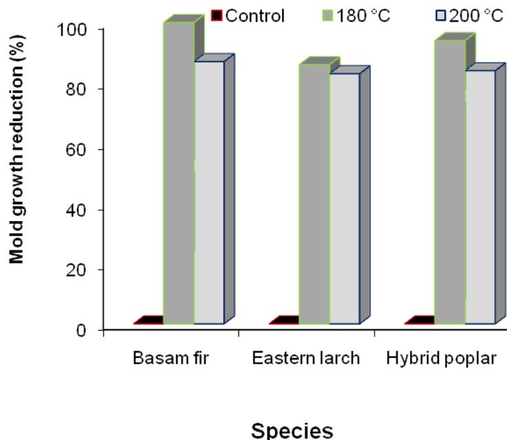
**Figure 3.** Effect of biothermal treatment on mould growth after 8 weeks of exposure on balsam fir, eastern larch and hybrid poplar
