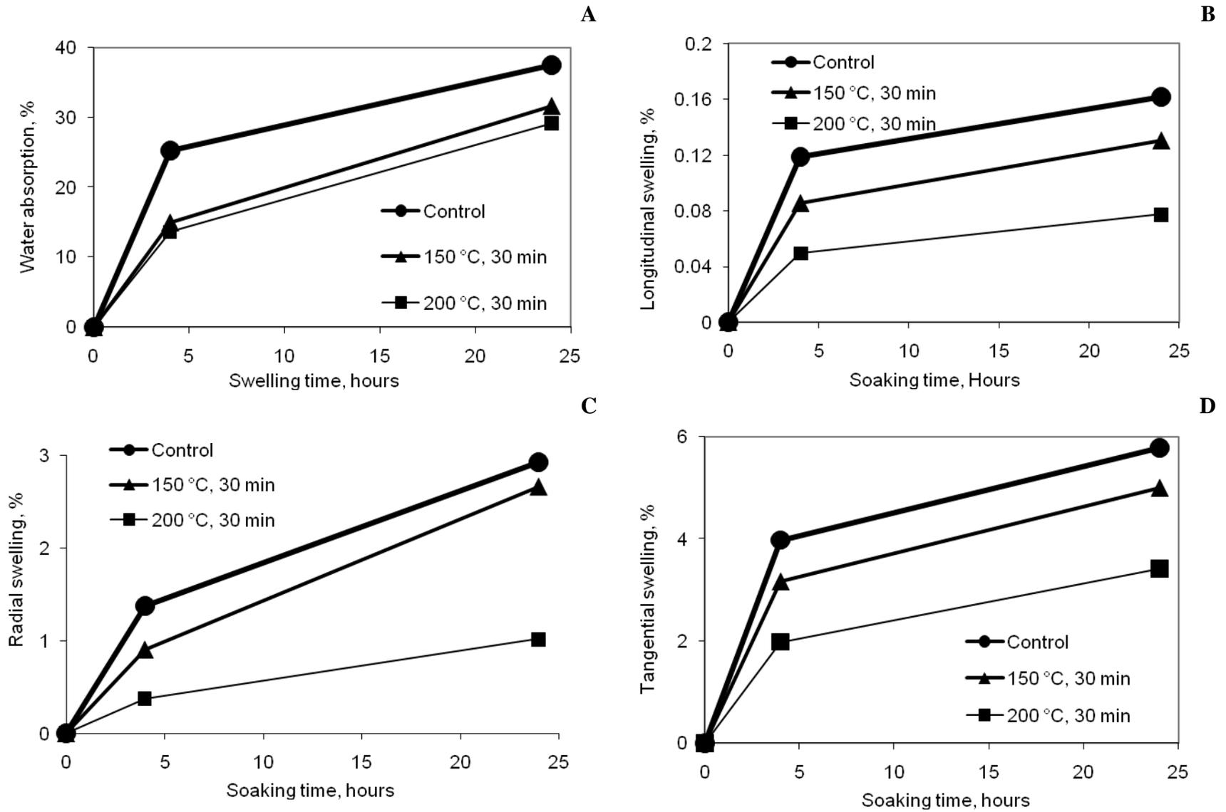
**Figure 1.** Impact of biothermal treatment on A. Water absorption; B. Longitudinal swelling; C. Radial swelling; and D. Tangential swelling for balsam fir (*Abies balsamea*)
