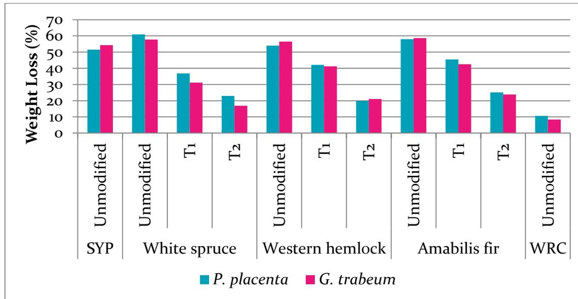
Figure 1: Weight loss in thermally modified samples exposed to two brown-rot fungi
