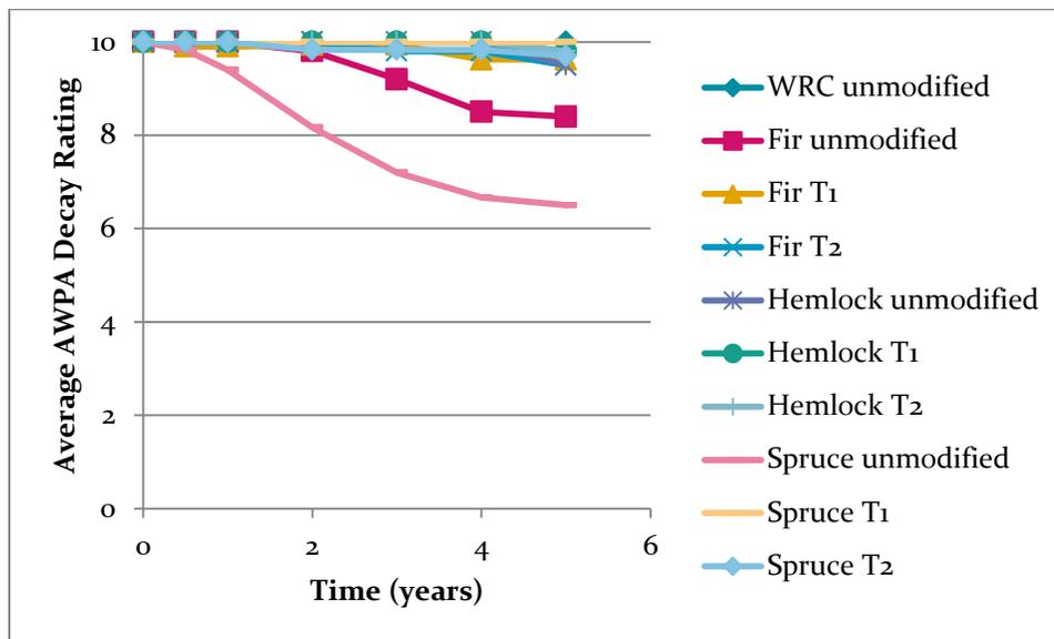
**Figure 2: Average AWP Decay Ratings of Materials Exposed in the Accelerated Field Simulator with only Spore Inoculum**
