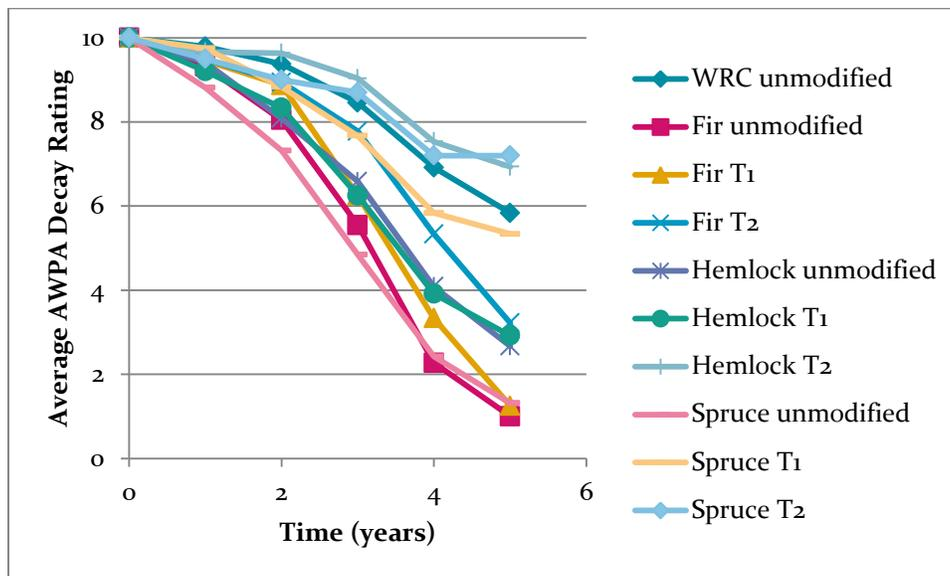
**Figure 5: Average AWPA Decay Ratings of Materials Exposed in AWPA E7 Stake Test**
