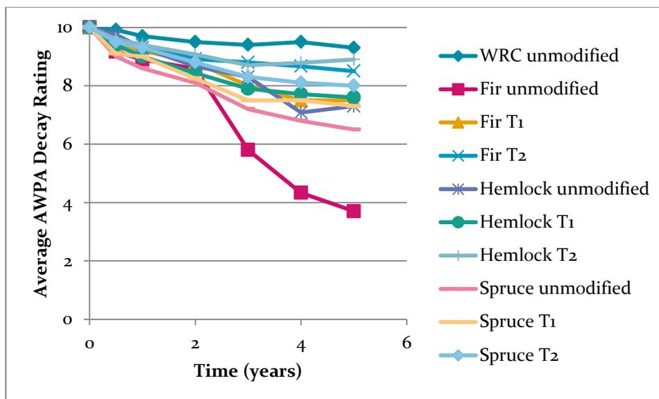
**Figure 3: Average AWP Decay Ratings of Materials Exposed in the Accelerated Field Simulator with Mycelial and Spore Inoculum**
