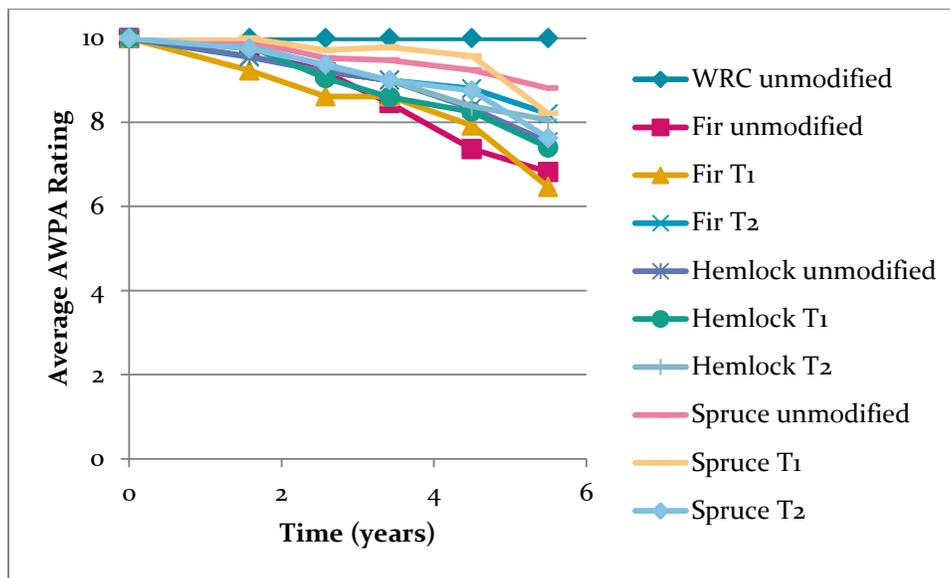
Figure 4: Average AWPA Decay Ratings of Materials Exposed in AWPA E9 L-Joint Test
