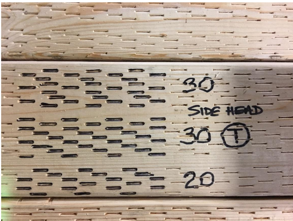
Figure 7 – 15ST Side Head Pattern used on the GenII Incisor identified as “T”
