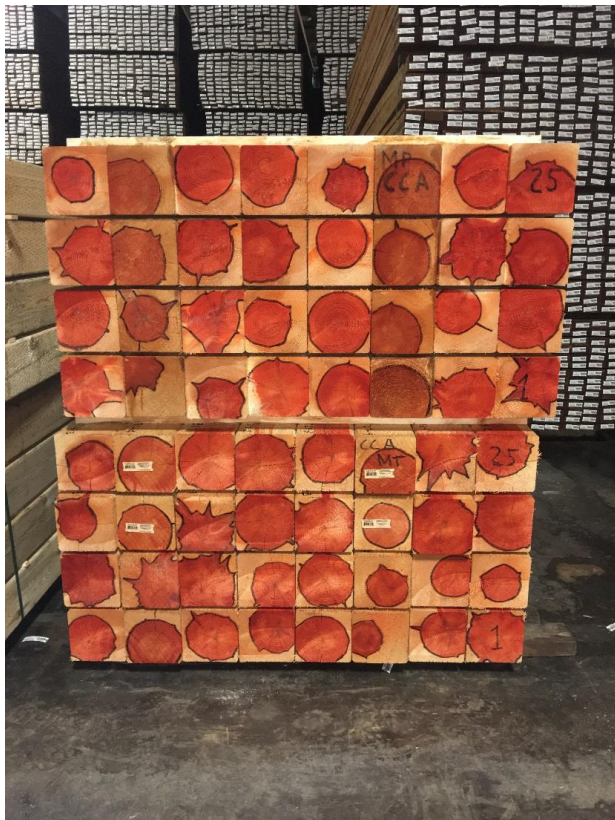
Figure 10 – CCA Michigan Red Pine Sprayed with Heartwood-Sapwood reagent and outlined with Marker
