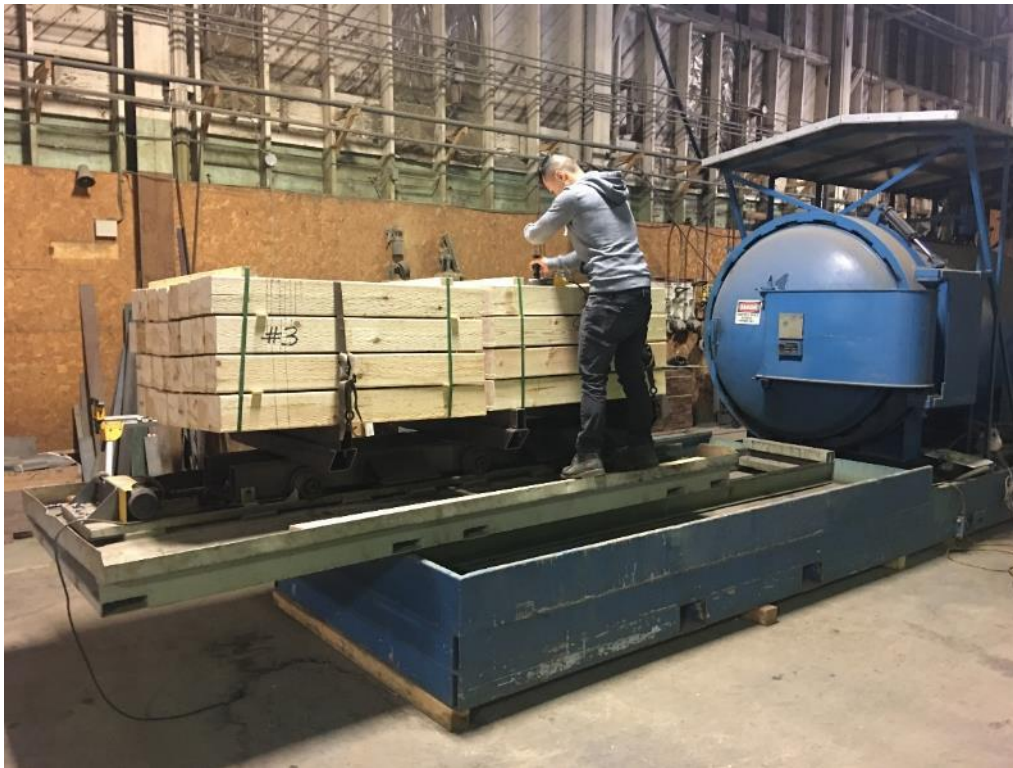
Figure 6 – Moisture Content Readings being taken with electrical resistance moisture meter prior to treatment in MicroOne
