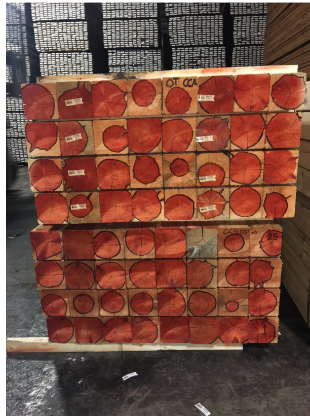
Figure 11 – CCA Ontario Sprayed with Heartwood-Sapwood reagent and outlined with Marker.
