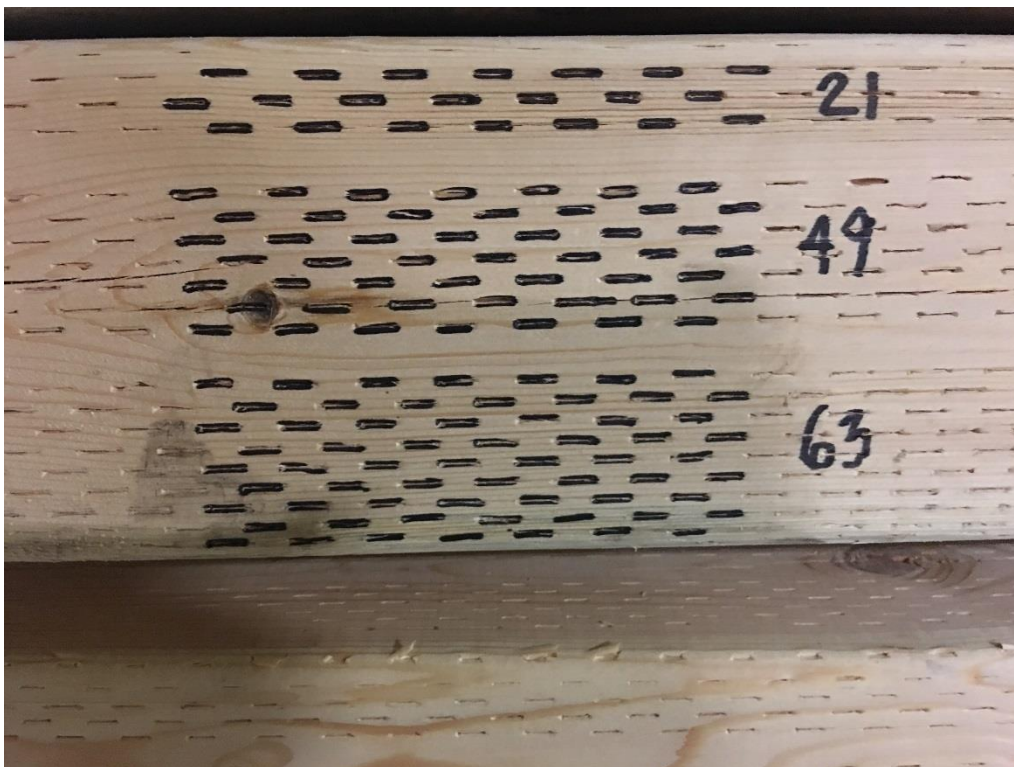
Figure 9 – 16ST Incising Pattern Pattern of the RJH Incisor identified as “p”
