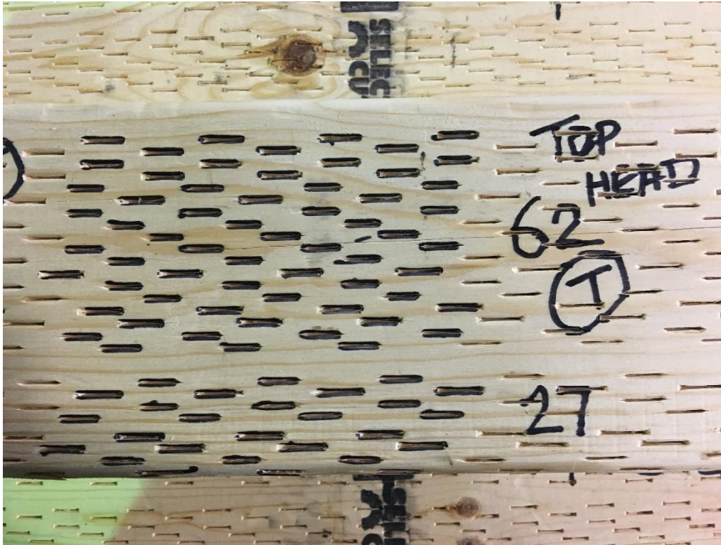
Figure 8 – 15ST Top Head Pattern on the GenII Incisor identified as “T”
