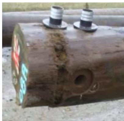
Figure 2. Metal sleeves used in the study on top and bottom end of holes
